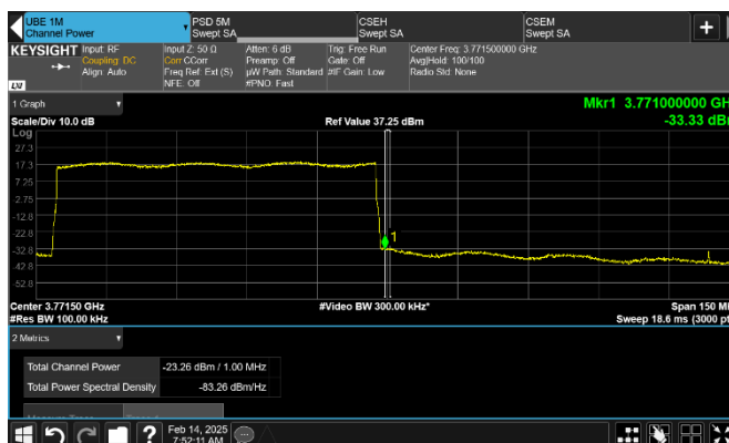
Figure 8.2-223: Conducted emission 1 MHz away from the upper frequency block edge of low channel
