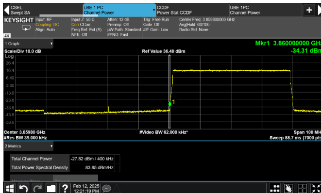
Figure 8.2-194: Conducted emission at the lower frequency block edge of top channel [ISED]
