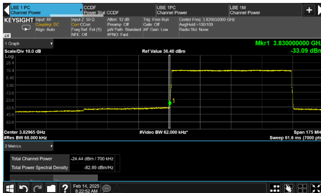
Figure 8.2-230: Conducted emission at the lower frequency block edge of top channel [ISED]
