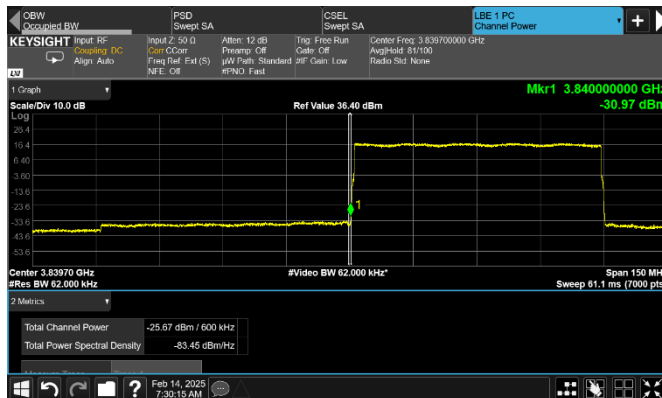
Figure 8.2-218: Conducted emission at the lower frequency block edge of top channel [ISED]
