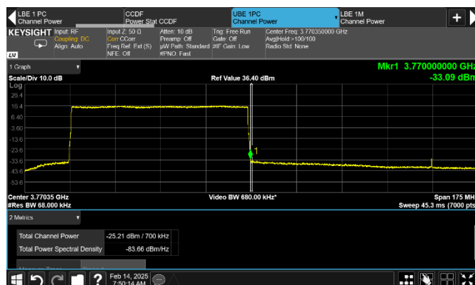
Figure 8.2-222: Conducted emission at the upper frequency block edge of low channel
