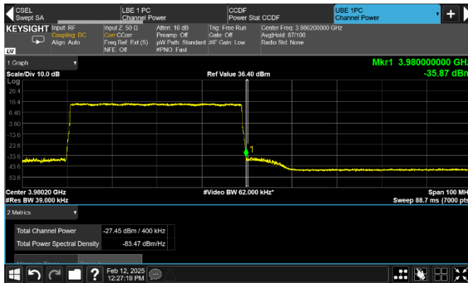
Figure 8.2-188: Conducted emission at the upper band edge
