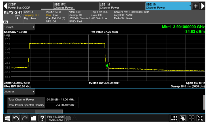
Figure 8.2-217: Conducted emission 1 MHz away from the upper band edge [ISED]
