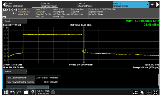
Figure 8.2-235: Conducted emission 1 MHz away from the upper frequency block edge of low channel
