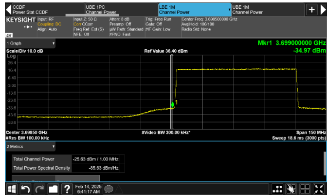
Figure 8.2-209: Conducted emission 1 MHz away from the lower band edge
