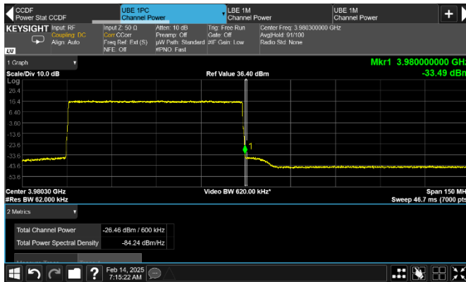
Figure 8.2-212: Conducted emission at the upper band edge
