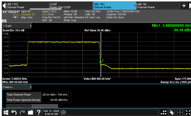
Figure 8.2-224: Conducted emission at the upper band edge
