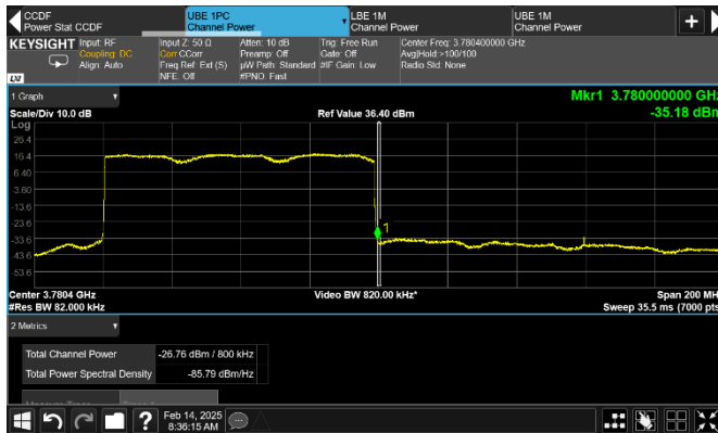
Figure 8.2-234: Conducted emission at the upper frequency block edge of low channel
