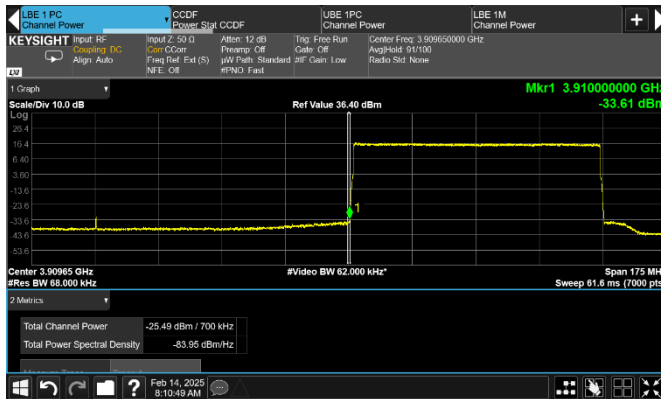
Figure 8.2-226: Conducted emission at the lower frequency block edge of top channel
