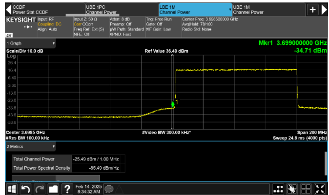
Figure 8.2-233: Conducted emission 1 MHz away from the lower band edge
