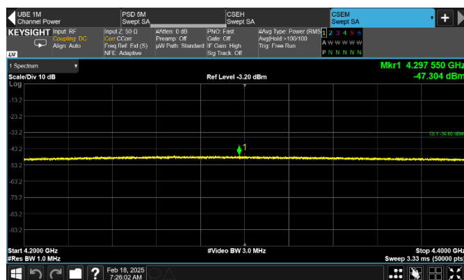
Figure 8.2-149: Conducted spurious emissions 4200 to 4400 MHz of NR 30 MHz six contiguous low channels, six-carrier operation
