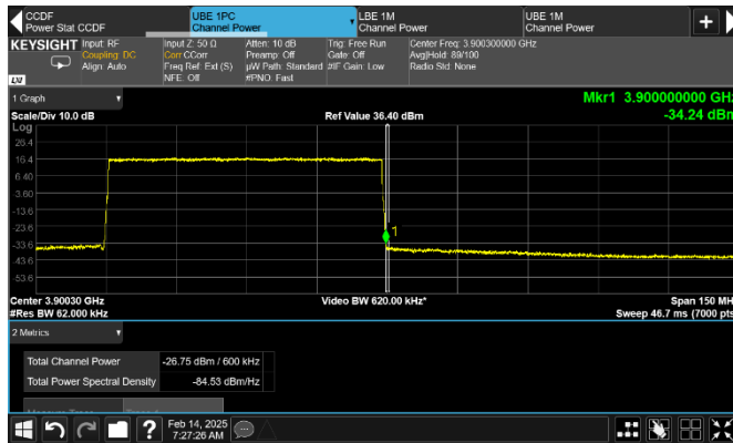
Figure 8.2-216: Conducted emission at the upper band edge [ISED]
