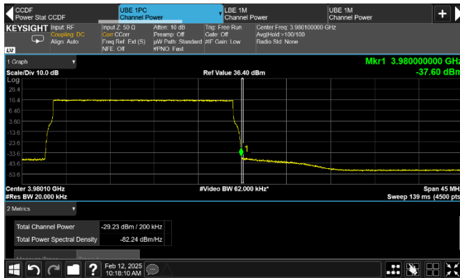
Figure 8.2-164: Conducted emission at the upper band edge
