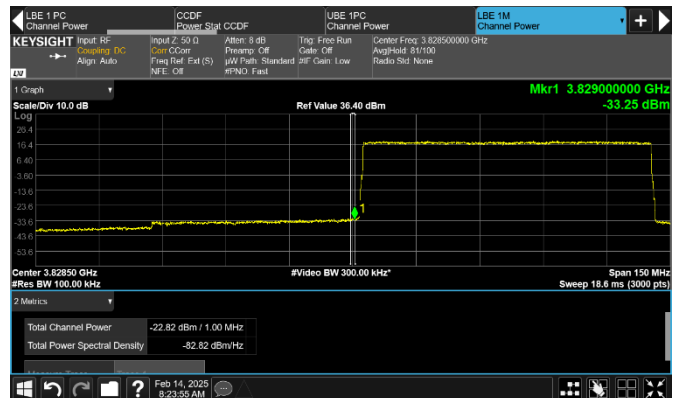
Figure 8.2-231: Conducted emission 1 MHz away from the lower frequency block edge of top channel [ISED]
