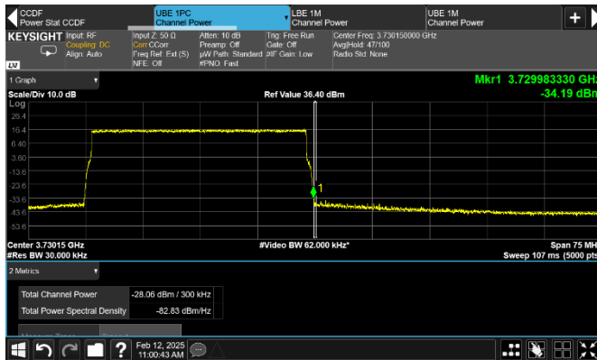
Figure 8.2-174: Conducted emission at the upper frequency block edge of low channel
