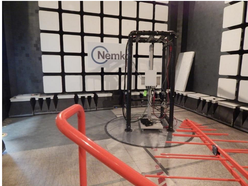
Figure-3: EUT Set-up photos for Radiated Emissions below 1 GHz
