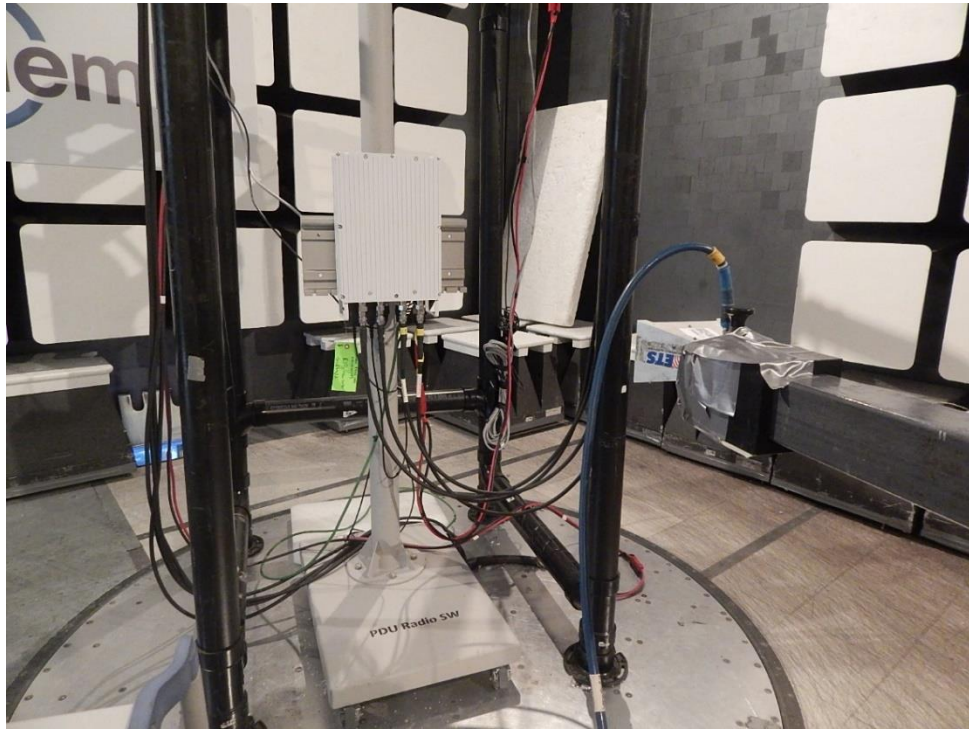
Figure-5: EUT Set-up photos for Radiated Emissions from 18-40 GHz
