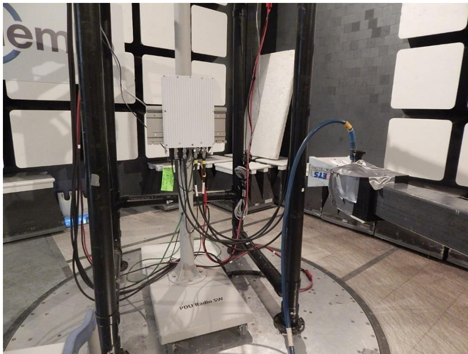
Figure 3.5-5: EUT Set-up photos for Radiated Emissions from 18-40 GHz
