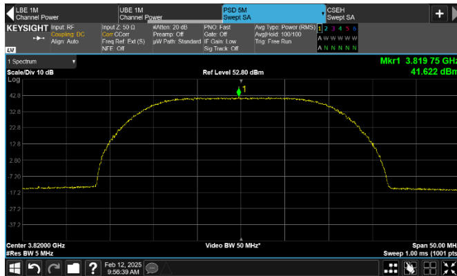
Figure 8.1-16: PSD of NR 20 MHz channel bandwidth, single carrier operation, sample plot (5 MHz Resolution)
