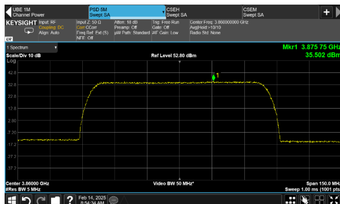
Figure 8.1-22: PSD of NR 80 MHz channel bandwidth, single carrier operation, sample plot (5 MHz Resolution)
