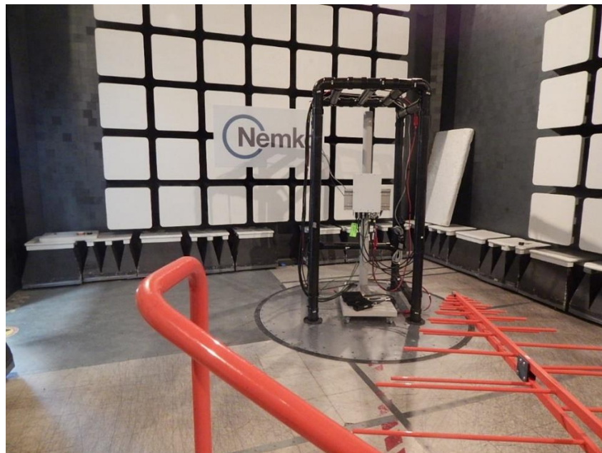
Figure 3.5-3: EUT Set-up photos for Radiated Emissions below 1 GHz
