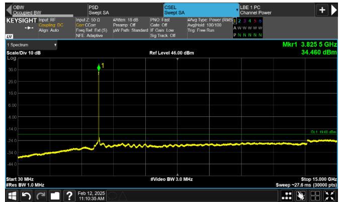
Figure 8.2-6: Conducted spurious emissions 30 MHz to 15 GHz of NR 30 MHz mid channel, single carrier operation
