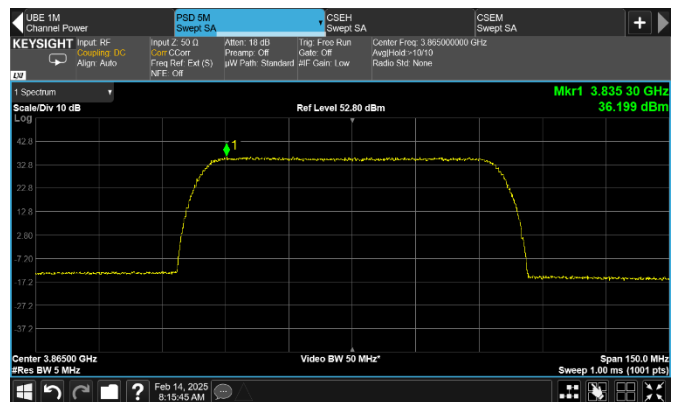
Figure 8.1-21: PSD of NR 70 MHz channel bandwidth, single carrier operation, sample plot (5 MHz Resolution)
