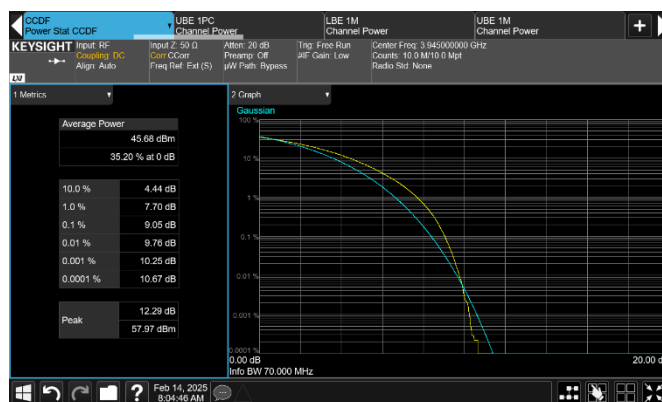
Figure 8.1-36: CCDF sample plot, NR 70 MHz
