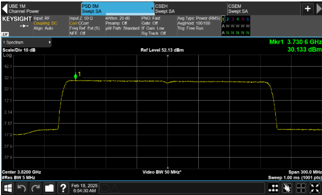
Figure 8.1-28: PSD of NR 100 MHz channel bandwidth, 2-carrier operation, sample plot (5 MHz Resolution)
