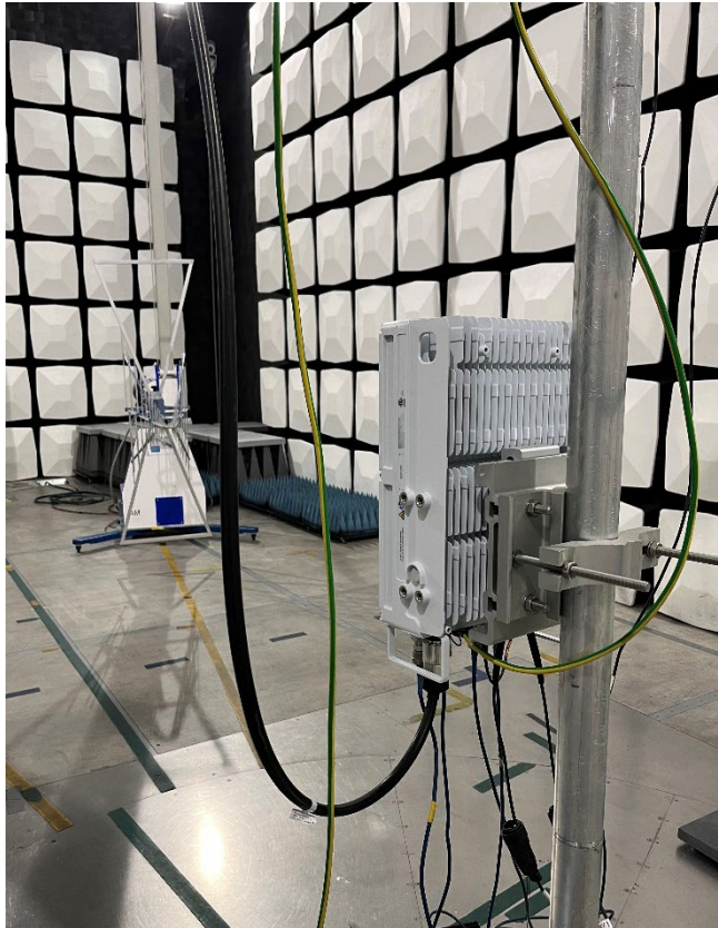
Photo of the test setup 30 – 1000 MHz
