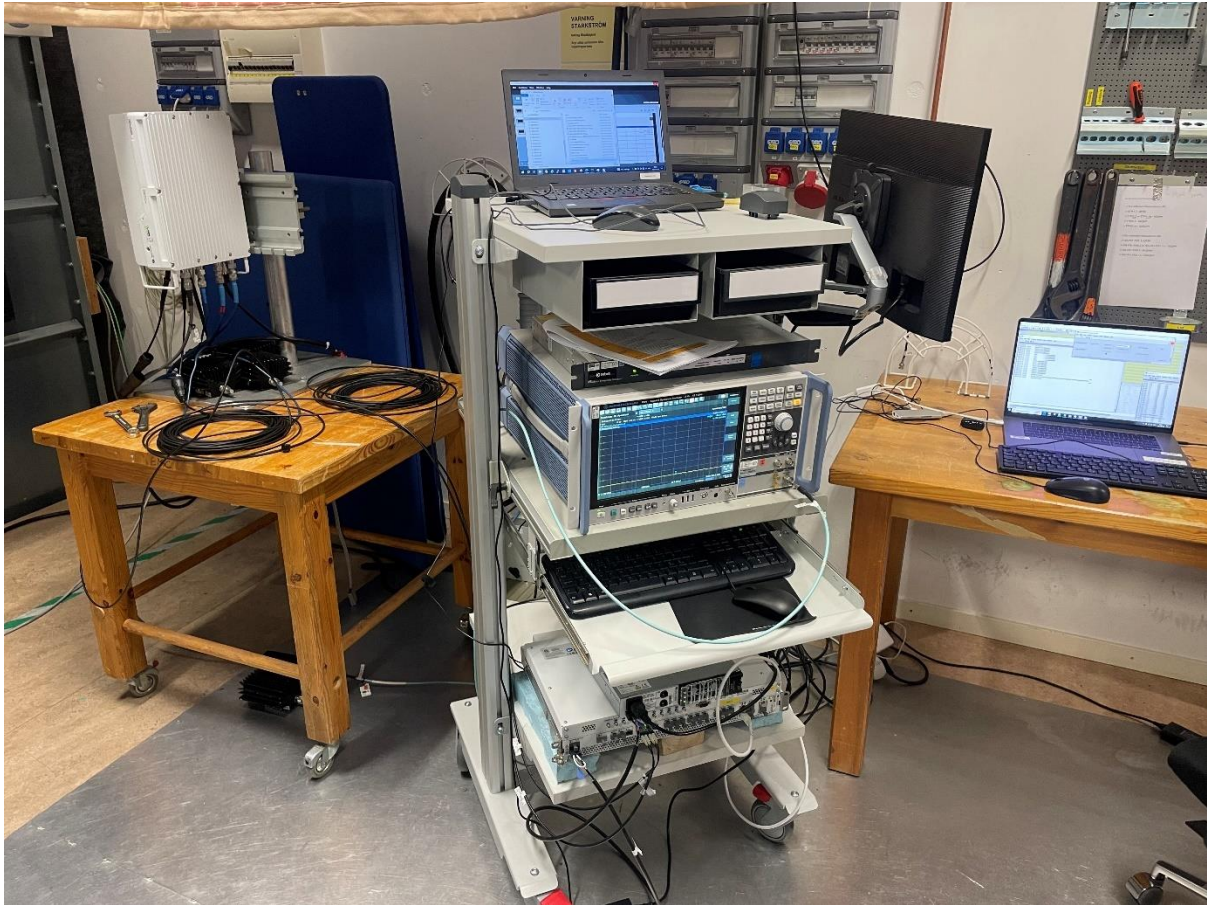
Test set-up for conducted measurements
