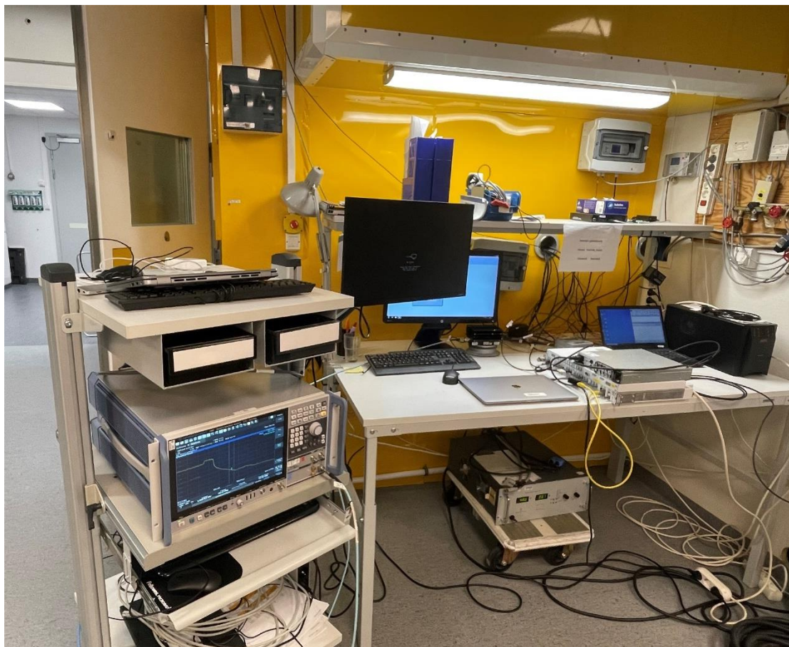
Test set-up for frequency stability (Outside the climate chamber)
