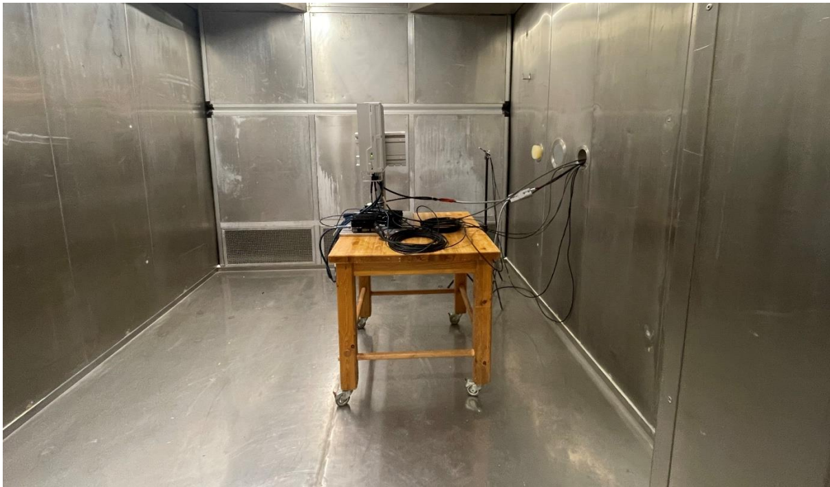
Test set-up for frequency stability (Inside the climate chamber)
