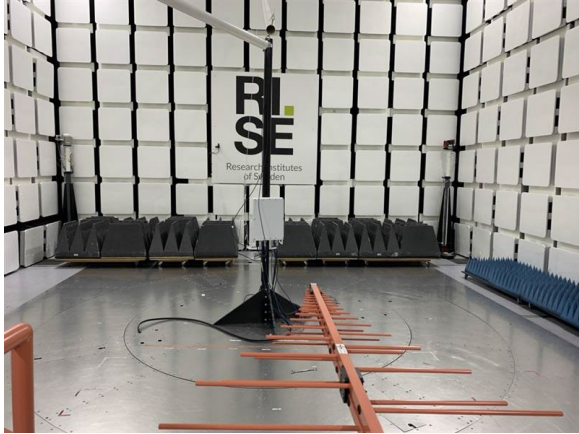
Test setup 30-1000 MHz:
