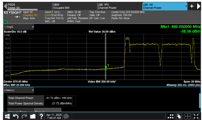
Figure 8.2-498: Conducted emission of 100 kHz at lower frequency block edge for top channel
