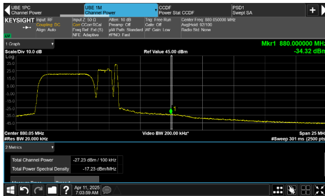
Figure 8.2-473: Conducted emission of 100 kHz at upper frequency block edge for low channel
