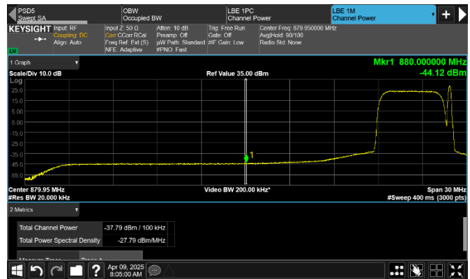
Figure 8.2-414: Conducted emission of 100 kHz at lower frequency block edge for top channel
