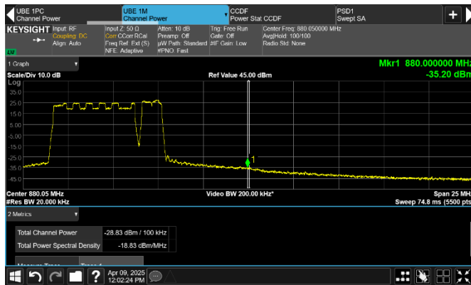
Figure 8.2-449: Conducted emission of 100 kHz at upper frequency block edge for low channel
