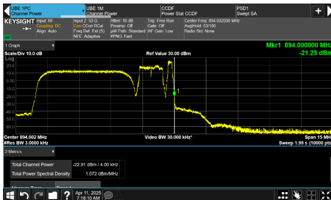
Figure 8.2-471: Conducted emission at the upper band edge
