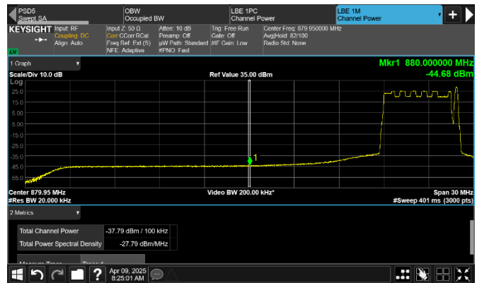
Figure 8.2-426: Conducted emission of 100 kHz at lower frequency block edge for top channel
