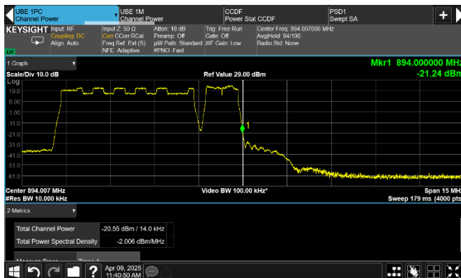
Figure 8.2-447: Conducted emission at the upper band edge
