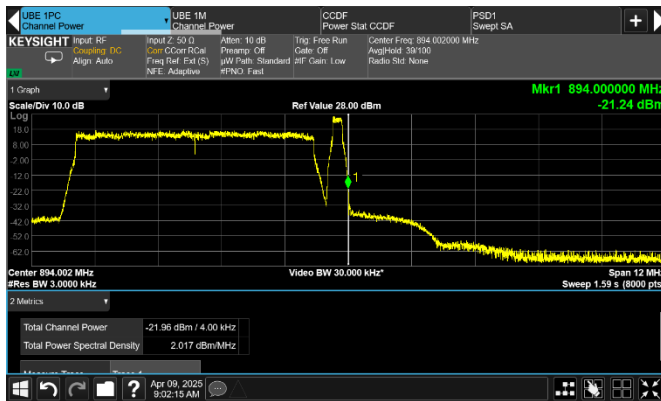
Figure 8.2-453: Conducted emission at the upper band edge
