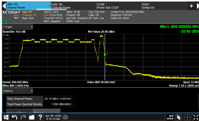
Figure 8.2-459: Conducted emission at the upper band edge
