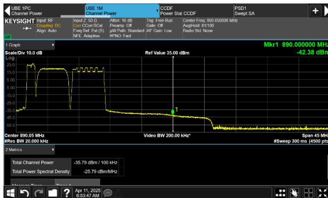
Figure 8.2-491: Conducted emission of 100 kHz at upper frequency block edge for low channel
