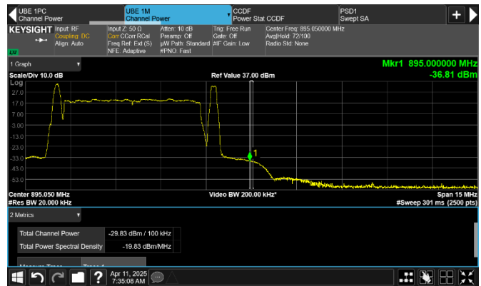
Figure 8.2-466: Conducted emission 1 MHz away from the upper band edge
