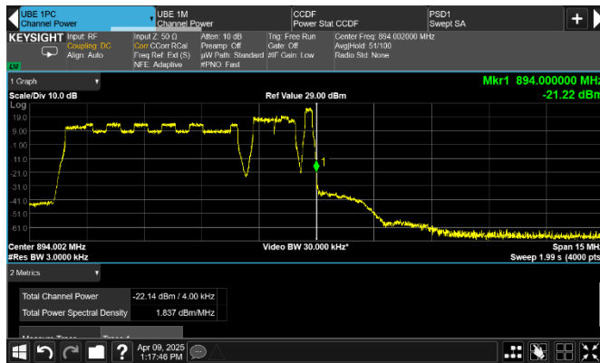
Figure 8.2-477: Conducted emission at the upper band edge
