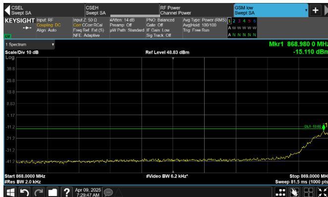
Figure 8.2-415: Conducted emission at the lower band edge
