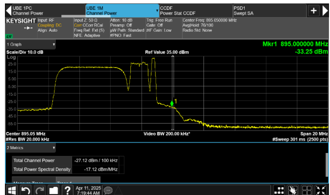
Figure 8.2-472: Conducted emission 1 MHz away from the upper band edge
