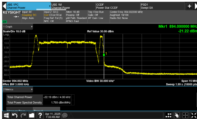
Figure 8.2-465: Conducted emission at the upper band edge
