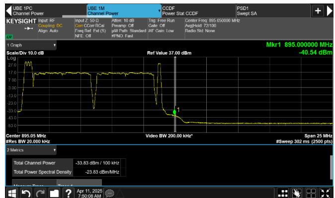
Figure 8.2-496: Conducted emission 1 MHz away from the upper band edge
