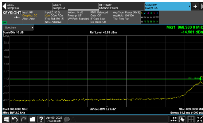
Figure 8.2-409: Conducted emission at the lower band edge
