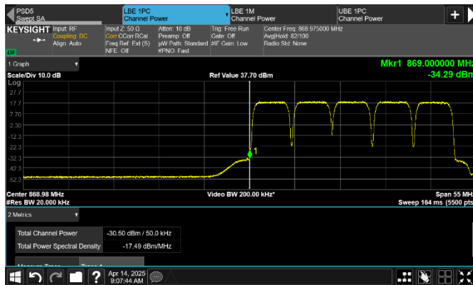
Figure 8.2-373: Conducted emission at the lower band edge
