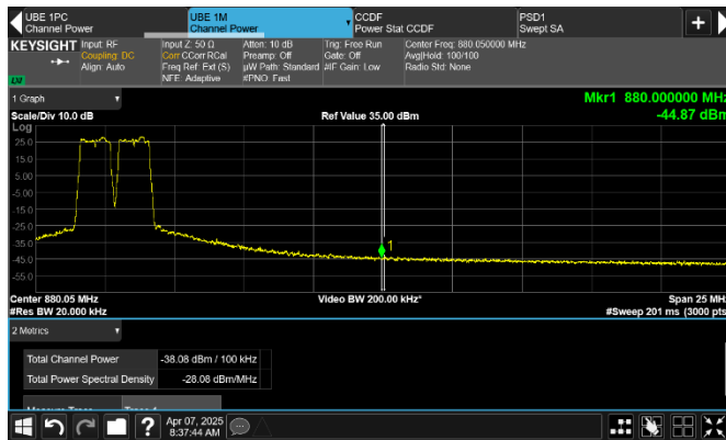
Figure 8.2-335: Conducted emission of 100 kHz at upper frequency block edge for low channel
