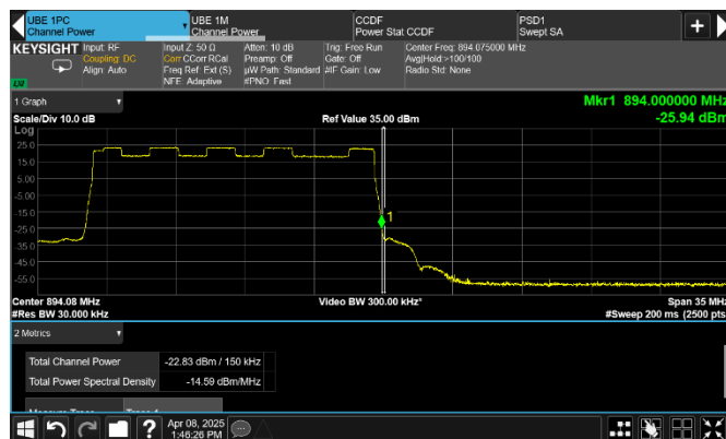
Figure 8.2-317: Conducted emission at the upper band edge
