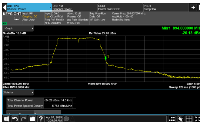
Figure 8.2-278: Conducted emission at the upper band edge
