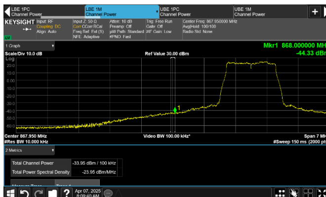
Figure 8.2-276: Conducted emission 1 MHz away from the lower band edge
