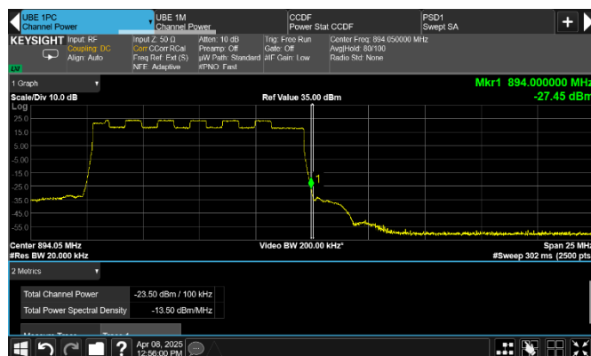
Figure 8.2-311: Conducted emission at the upper band edge
