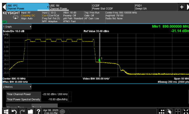
Figure 8.2-320: Conducted emission at upper frequency block edge for low channel
