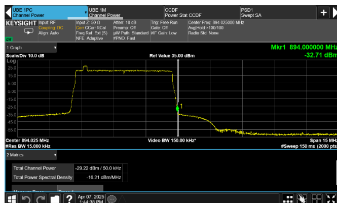
Figure 8.2-289: Conducted emission at the upper band edge
