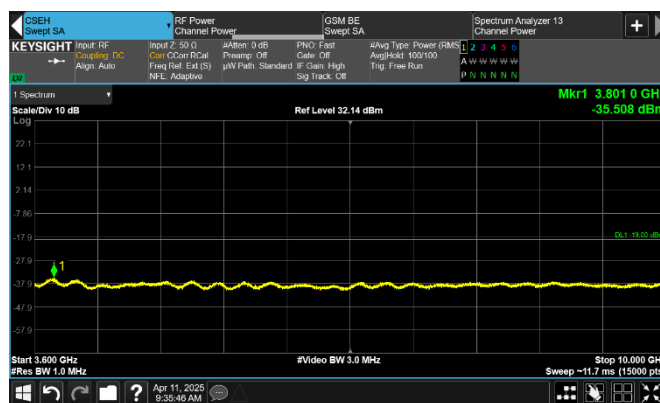
Figure 8.2-234: Conducted spurious emissions 3.6 GHz to 10 GHz of 2xLTE 1.4 MHz + 2xWCDMA + 2xNR 5 MHz six contiguous low channels, six carrier operation
