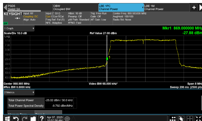
Figure 8.2-281: Conducted emission at the lower band edge
