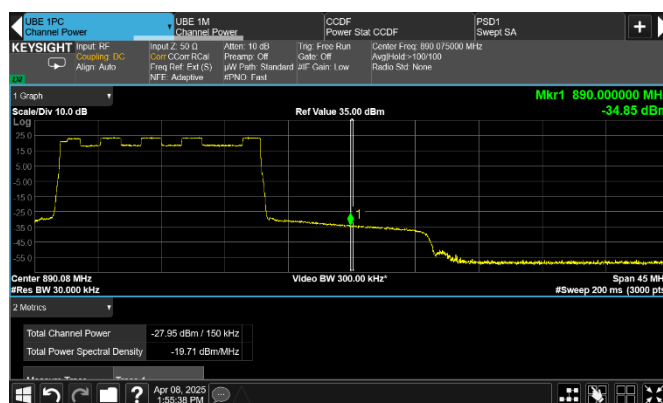
Figure 8.2-316: Conducted emission at upper frequency block edge for low channel
