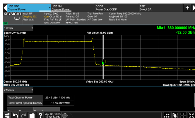
Figure 8.2-295: Conducted emission at the upper frequency block edge of the lower channel
