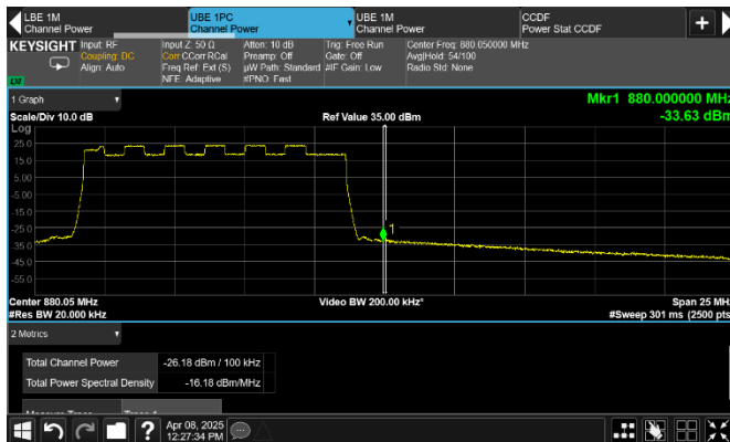
Figure 8.2-309: Conducted emission at the upper frequency block edge of the lower channel
