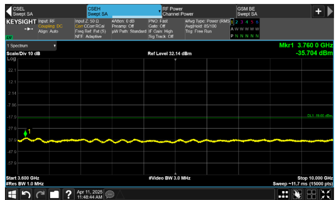
Figure 8.2-140: Conducted spurious emissions 3.6 GHz to 10 GHz of NR 5 MHz + GSM two contiguous mid channels, two carrier operation
