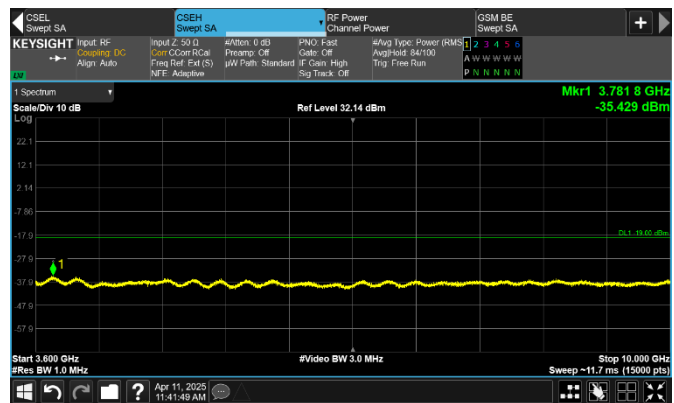
Figure 8.2-128: Conducted spurious emissions 3.6 GHz to 10 GHz of WCDMA + GSM two contiguous mid channels, two carrier operation
