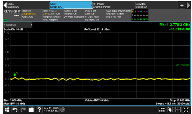
Figure 8.2-198: Conducted spurious emissions 3.6 GHz to 10 GHz of GSM + LTE 1.4 MHz + NR 5 MHz three contiguous low channels, 3-carrier operation
