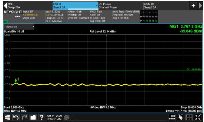
Figure 8.2-204: Conducted spurious emissions 3.6 GHz to 10 GHz of LTE 1.4 MHz + WCDMA + NR 5 MHz contiguous low channels, 3-carrier operation
