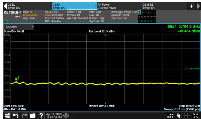
Figure 8.2-200: Conducted spurious emissions 3.6 GHz to 10 GHz of GSM + LTE 1.4 MHz + NR 5 MHz three contiguous mid channels, 3-carrier operation
