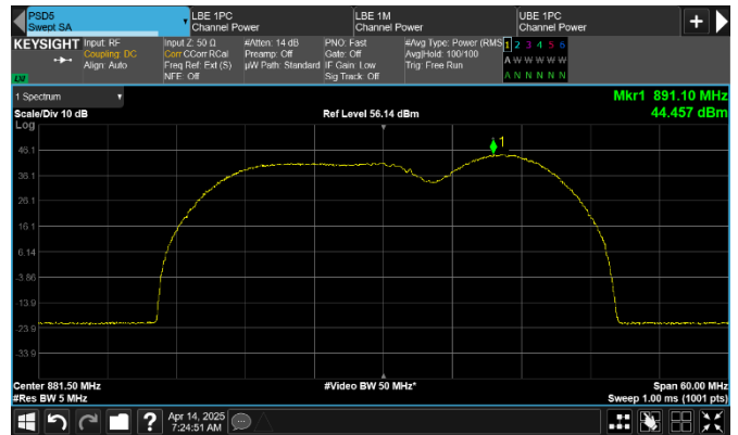
Figure 8.1-126: PSD of 2 x NR 5 MHz + IoT SA 0.4 + 3 x LTE 1.4 MHz, 6-carrier non-contiguous operation, sample plot (5 MHz Resolution)
