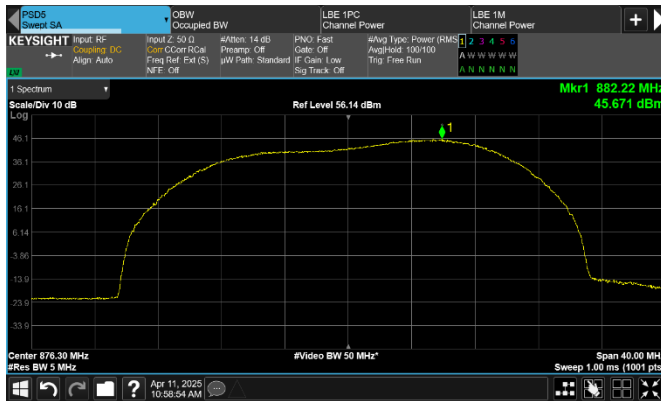
Figure 8.1-107: PSD of 2 x NR 5 MHz + 3 x LTE 1.4 MHz + IoT SA 0.4 MHz, 6-carrier operation, sample plot (5 MHz Resolution)
