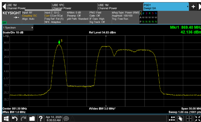
Figure 8.1-63: PSD of 2 x GSM 0.2 MHz + 2 x LTE 1.4 MHz + 2 x NR 5 MHz, 6-carrier non-contiguous operation, sample plot (1 MHz Resolution)
