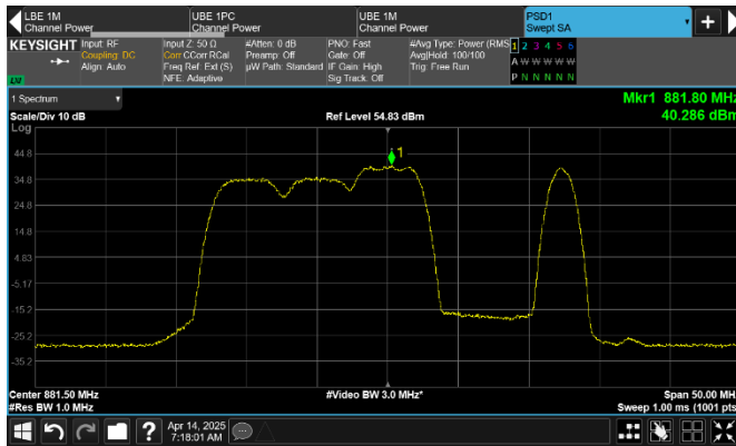
Figure 8.1-61: PSD of 2 x WCDMA 5 MHz + 3 x LTE 1.4 MHz + IoT SA 0.4 MHz, 6-carrier non-contiguous operation, sample plot (1 MHz Resolution)
