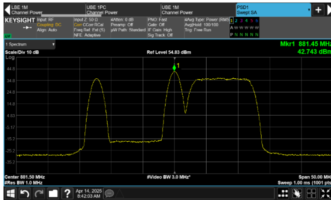
Figure 8.1-55: PSD of GSM 0.2 MHz + IoT SA 0.4 MHz + LTE 10 MHz, 3-carrier non-contiguous operation, sample plot (1 MHz Resolution)
