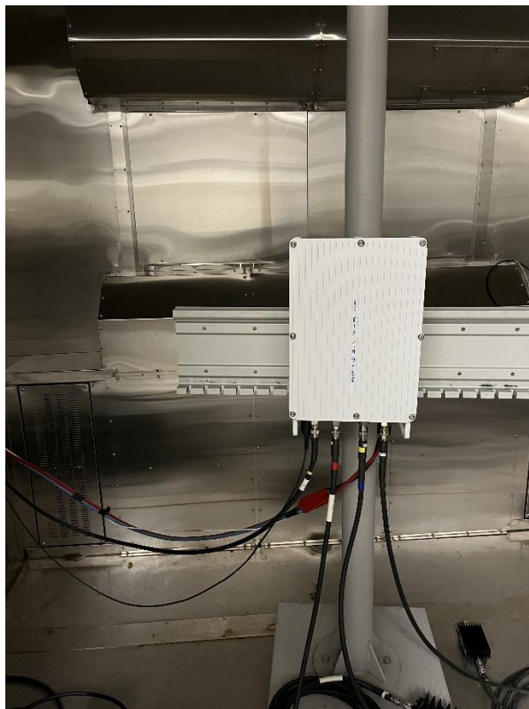
Figure 3.5-2: EUT Set-up photo for Thermal Radio Compliance Testing
