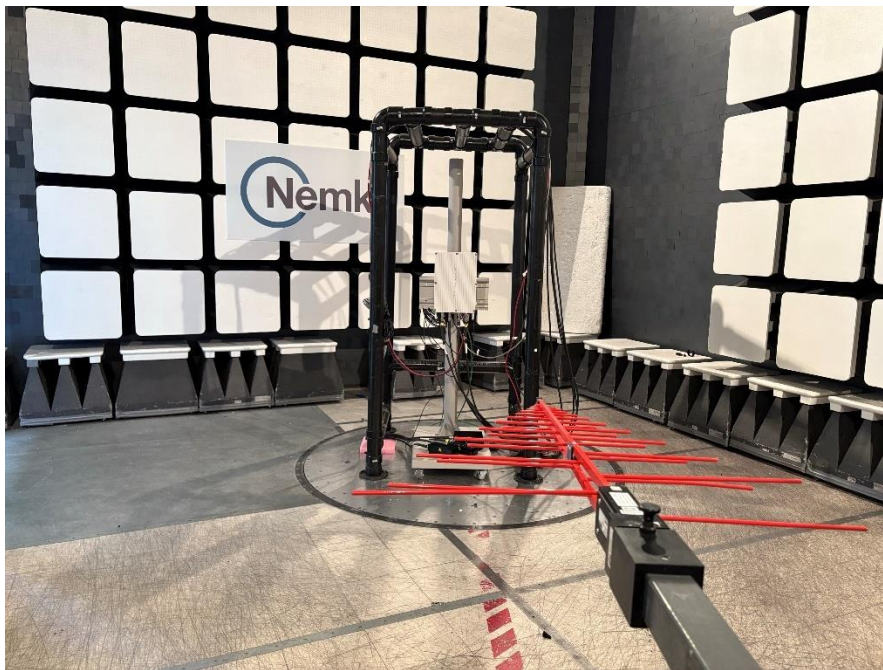
Figure 3.5-4: EUT Set-up photos for Cabinet Radiated Emissions 200 to 1000 MHz
