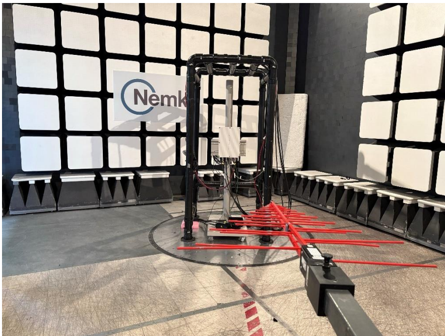
Figure o-4: EUT Set-up photos for Cabinet Radiated Emissions 200 to 1000 MHz
