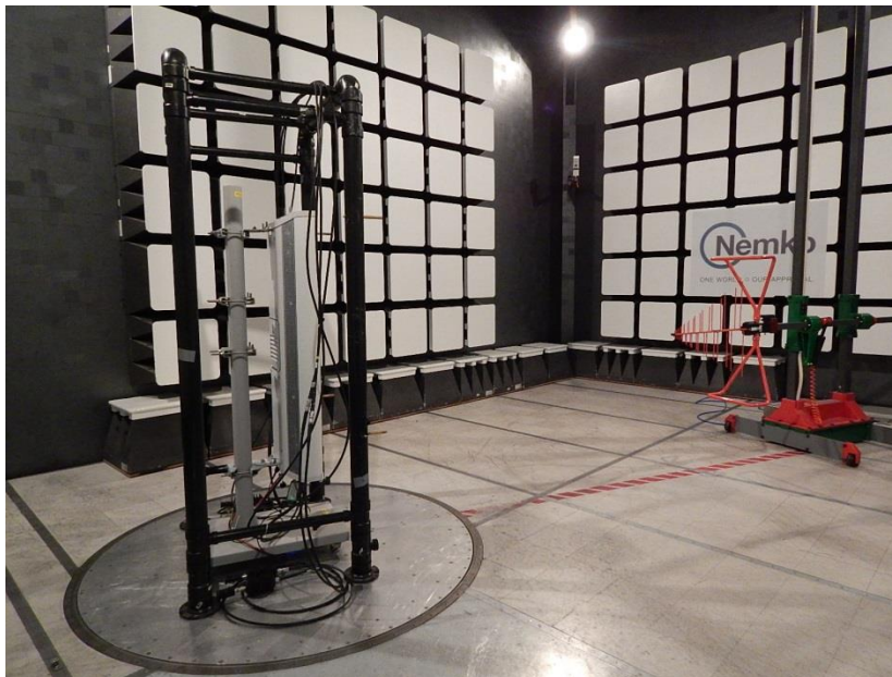
Figure 8.1-38: Setup photo – 30 to 1000 MHz
