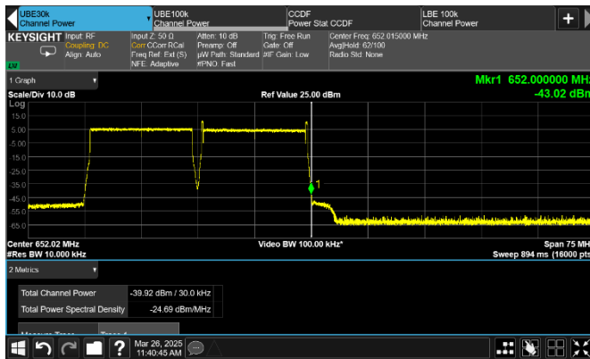
Figure 8.3-169: Conducted emission at the upper band edge
