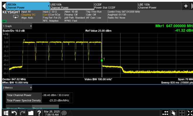
Figure 8.3-175: Conducted emission at the upper frequency block edge of low channel
