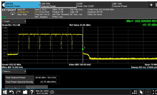
Figure 8.3-177: Conducted emission at the upper band edge
