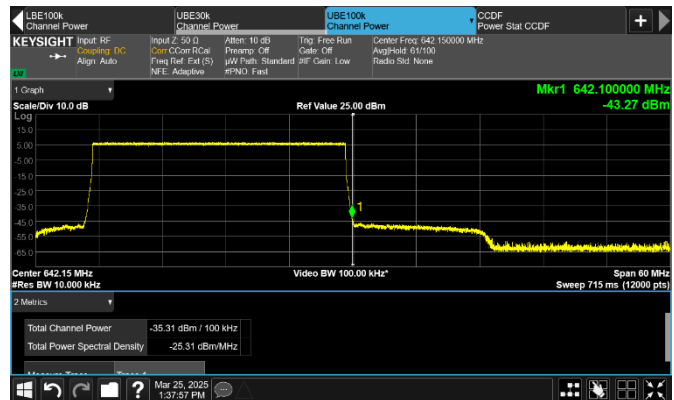
Figure 8.3-136: Conducted emission 100 kHz away from the upper frequency block edge of low channel
