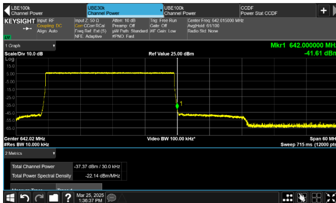
Figure 8.3-135: Conducted emission at the upper frequency block edge of low channel
