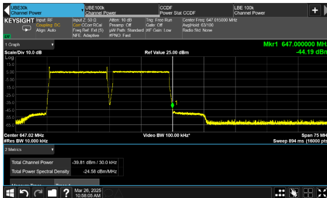
Figure 8.3-167: Conducted emission at the upper frequency block edge of low channel
