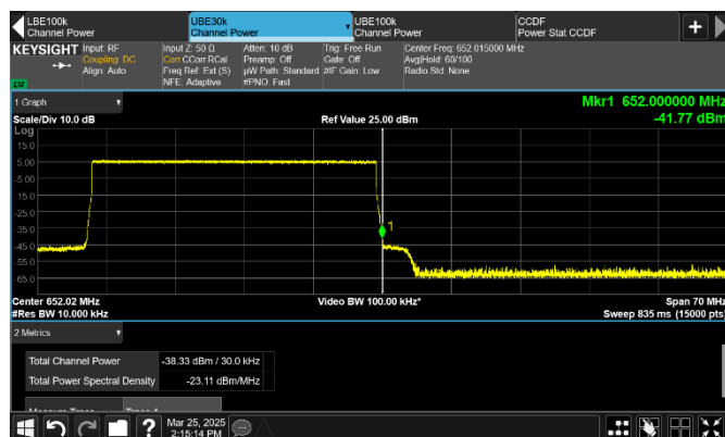
Figure 8.3-145: Conducted emission at the upper band edge
