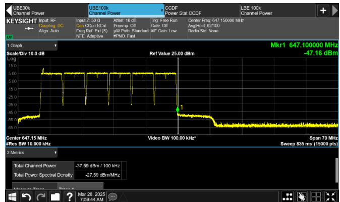
Figure 8.3-176: Conducted emission 100 kHz away from the upper frequency block edge of low channel
