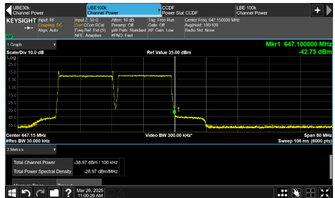
Figure 8.3-168: Conducted emission 100 kHz away from the upper frequency block edge of low channel
