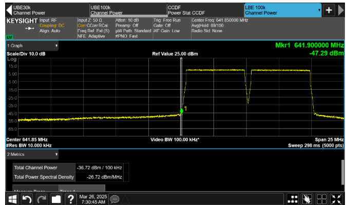
Figure 8.3-188: Conducted emission 100 kHz away from the lower frequency block edge of top channel
