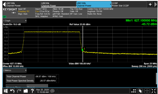
Figure 8.3-112: Conducted emission 100 kHz away from the upper frequency block edge of low channel
