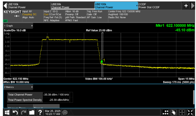
Figure 8.3-72: Conducted emission 100 kHz away from the upper frequency block edge of low channel
