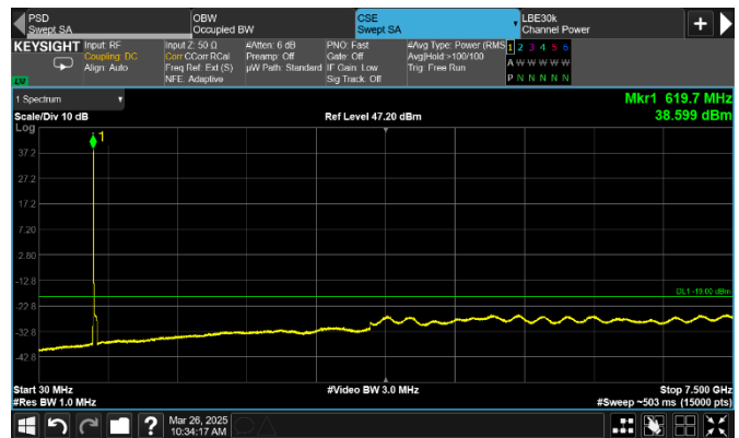
Figure 8.3-16: Conducted spurious emissions of NR 5 MHz low channel, single carrier operation
