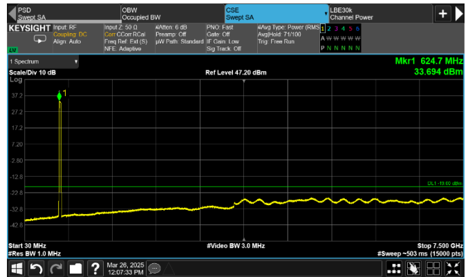
Figure 8.3-48: Conducted spurious emissions of 2 x NR 15 MHz mid channels, 2-carrier operation
