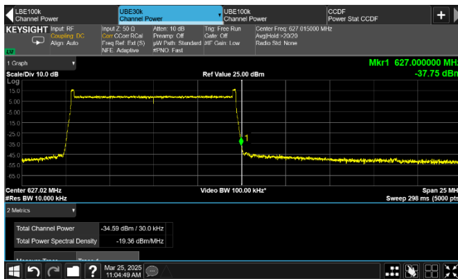
Figure 8.3-79: Conducted emission at the upper frequency block edge of low channel
