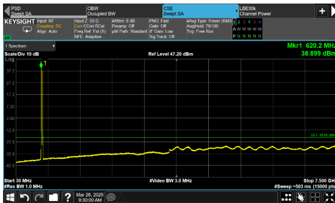
Figure 8.3-67: Conducted spurious emissions of LTE 5 MHz + IoT SA channels, 2-carrier operation [Non-contiguous]
