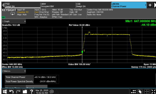
Figure 8.3-75: Conducted emission at the lower frequency block edge of top channel
