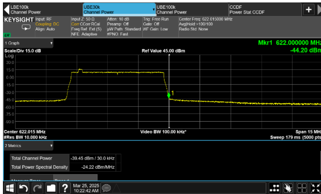
Figure 8.3-71: Conducted emission at the upper frequency block edge of low channel
