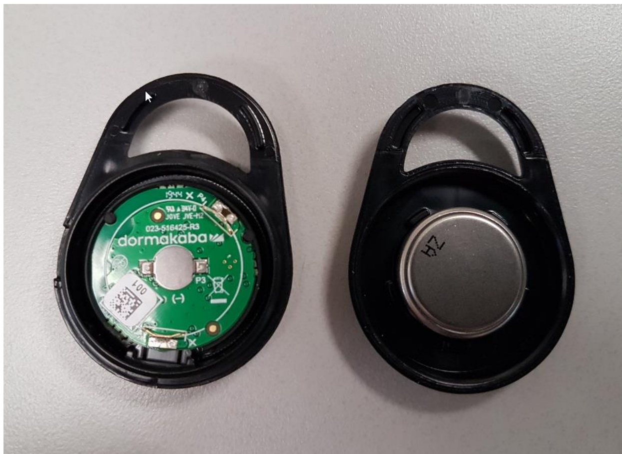
Figure 1- Open Fob with PCB and coin cell battery inside
