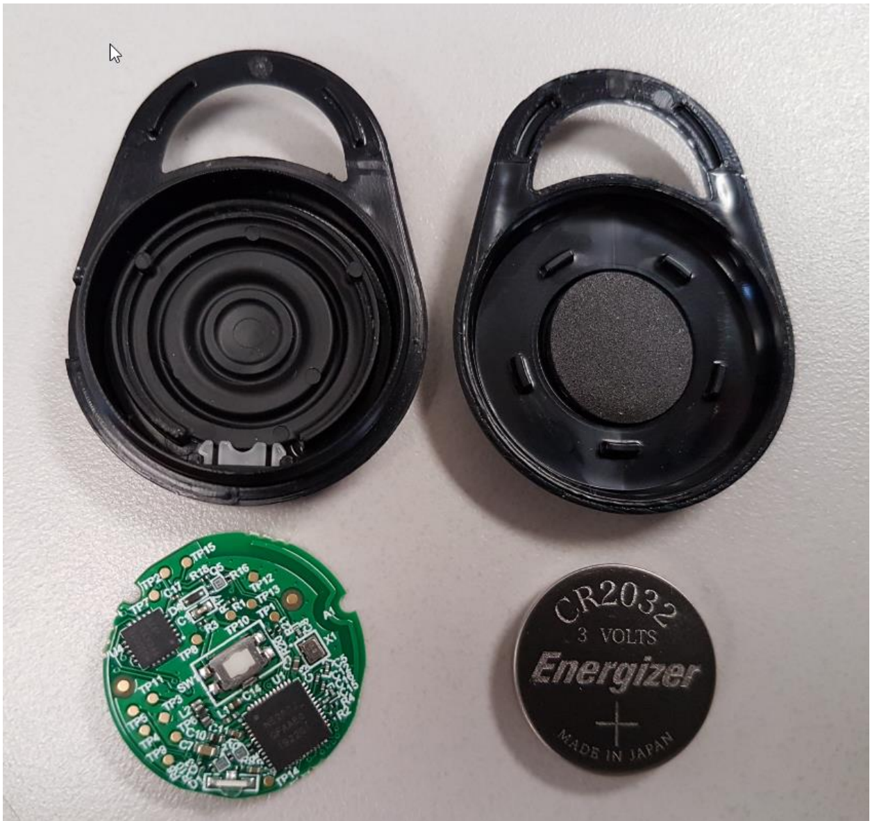
Figure 2- Open Fob with PCB and coin cell battery removed
