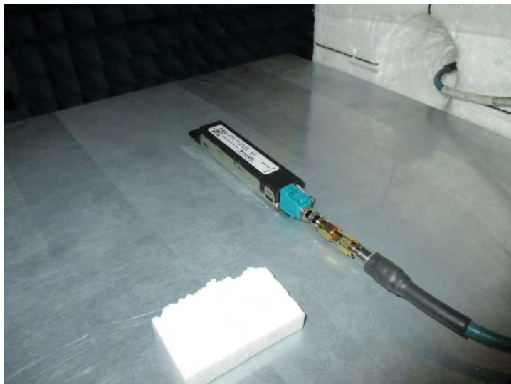
The 85H 035 225 B Amplifier on 35x35 cm ground plane/metal plate in the Proant anechoic chamber
