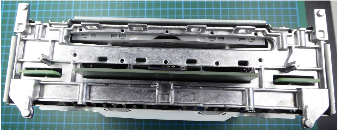
160090_17. jpg: EUT – Main Unit without front panel – Front view
