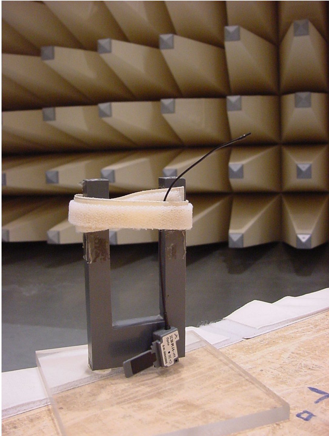
Photo 6 (Radiated Emissions): Tx with Lambda/4 antenna
