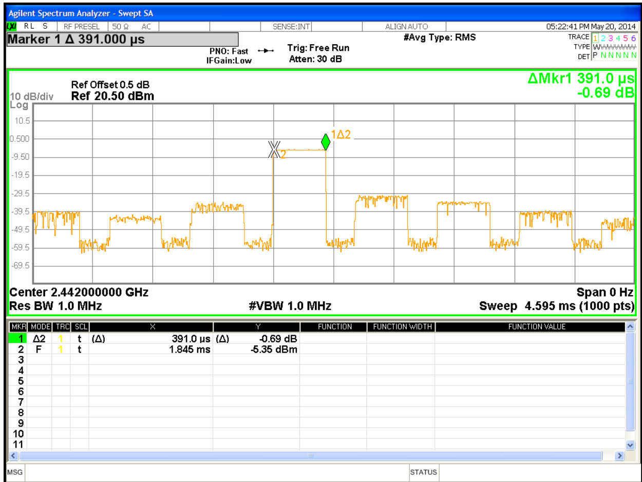
Figure 8: Pulse Width – Channel 2442MHz
