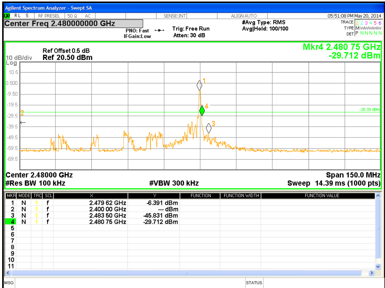
Figure 17: Band Edge Requirements at 2480 MHz
