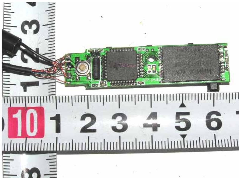
EUT – PCB View of Bluetooth Module
