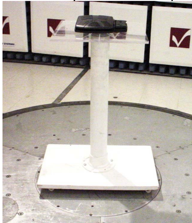
View of the EUT as positioned on the test pedestal
