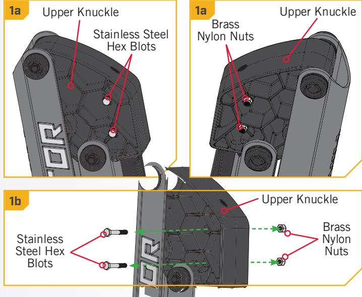
**NOTICE:** It may be necessary to use a socket extension or a deep socket because the Hex Bolts and Brass Nylon Nuts are recessed into the Upper Knuckle.
