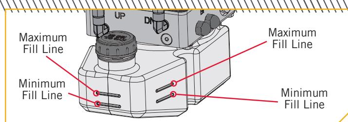
Note the color of the hydraulic fluid. If over time the hydraulic fluid becomes discolored, it may be a sign of contamination. Change the fluid and check the seal on the Pump Reservoir, the seal between the Hydraulic Hoses and the Hydraulic fittings on the Manifold and the Hydraulic Hoses and the Hydraulic Cylinder on the anchor to ensure that the Hydraulic Circuit remains sealed.
