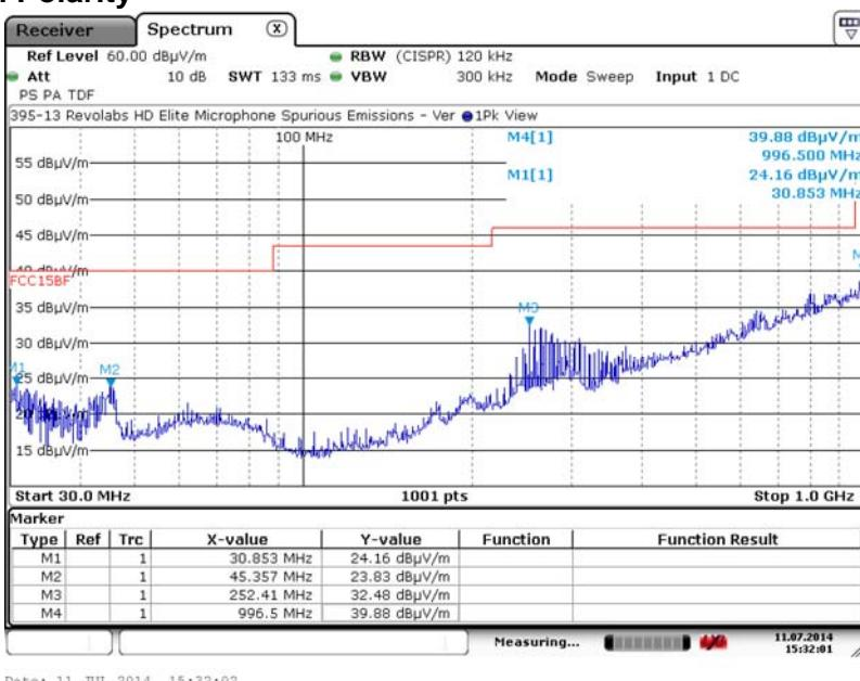
Prescan from Compact 3 Meter Chamber, no Measurable signals on 3 Meter OATS.
