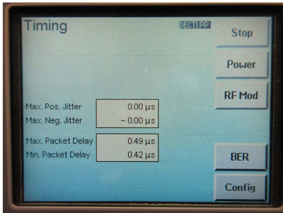
**Note:** The tester is configured for 1000 bursts of analysis (its maximum) and then monitored for a minimum of 1000 seconds recording the maximum and minimum values of jitter to satisfy the measurement requirement over 100,000 frames.
