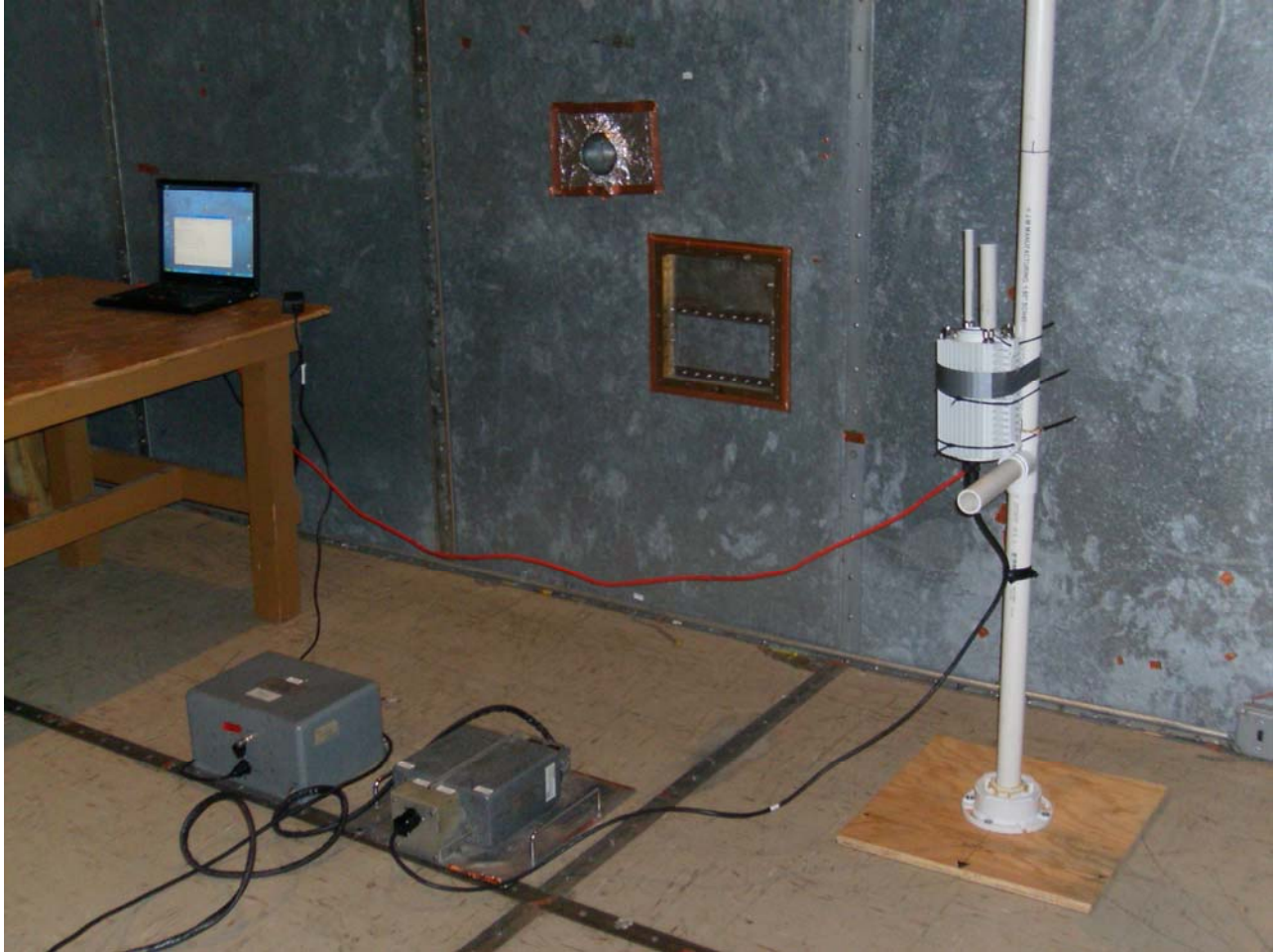
Photograph 2. Conducted Emissions Test Setup
