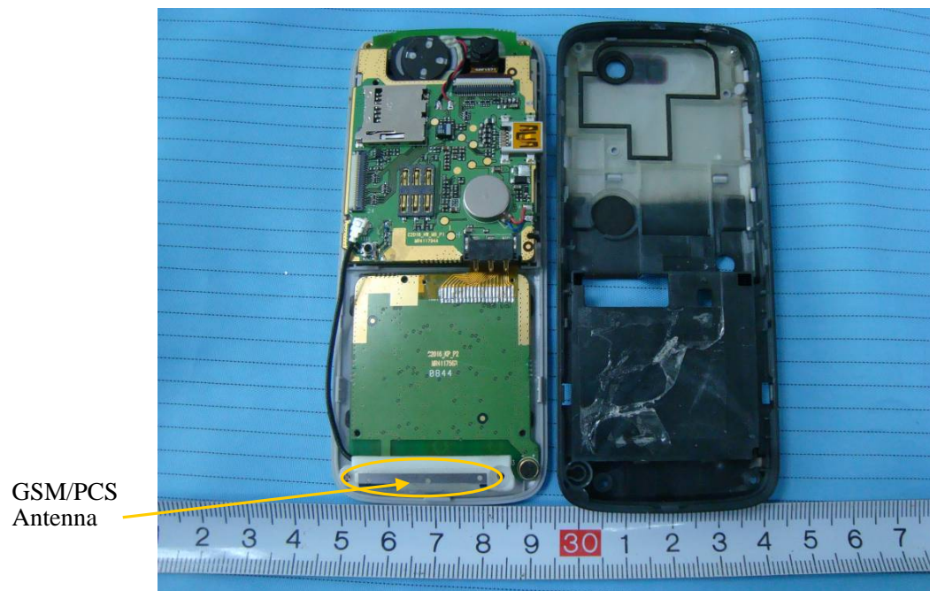
EUT – Uncovered Rear View
