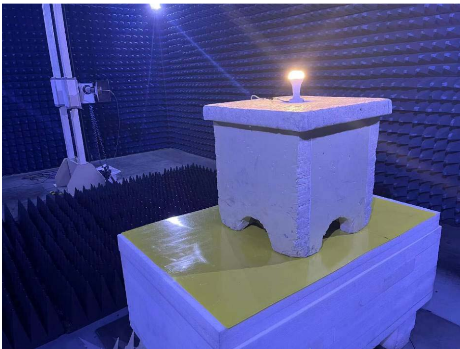
Photo of Radiated Emission Measurement Above 1GHz
