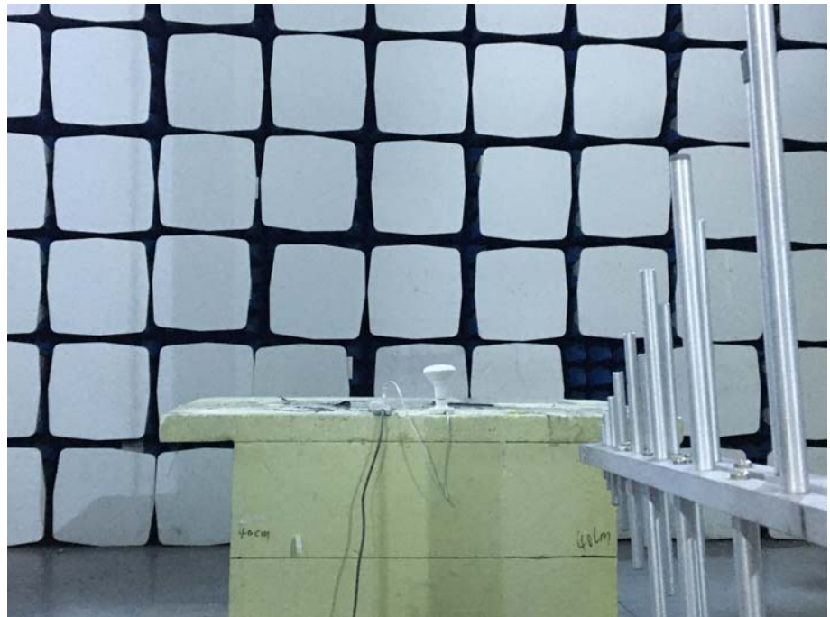
Radiation Emission Test Setup (30MHz to 1GHz)
