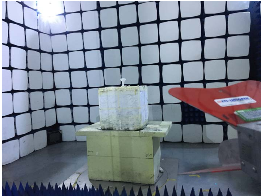
Radiation Emission Test Setup (1GHz to 18GHz)
