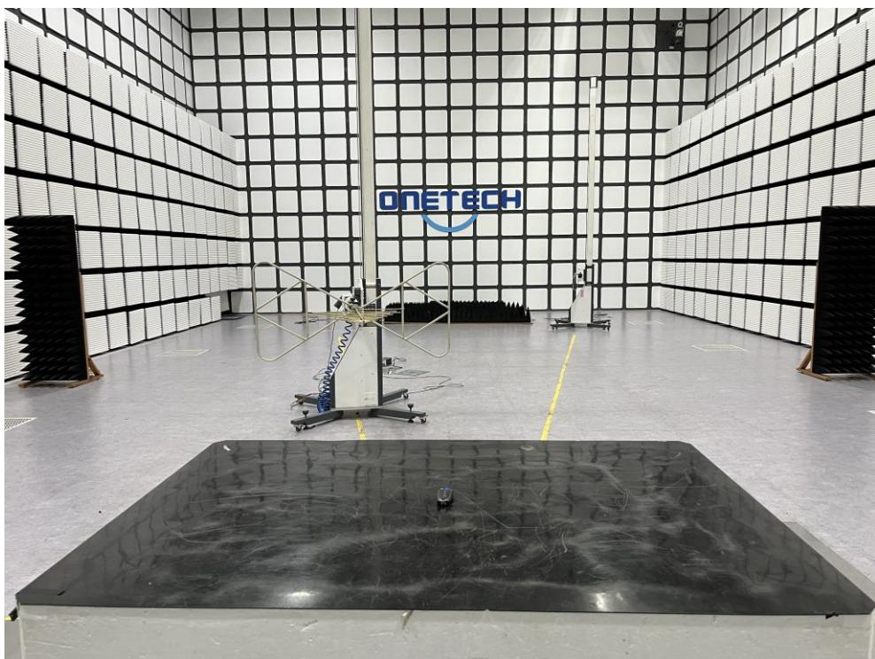
**- Radiated Emission Test (Above 1 GHz)**
