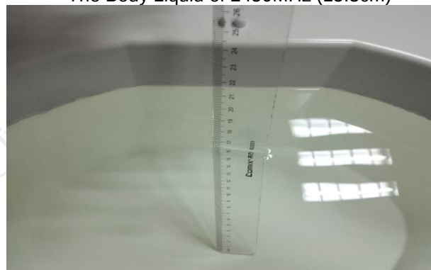
The Body Liquid of 5000-6000MHz (16.5cm)
