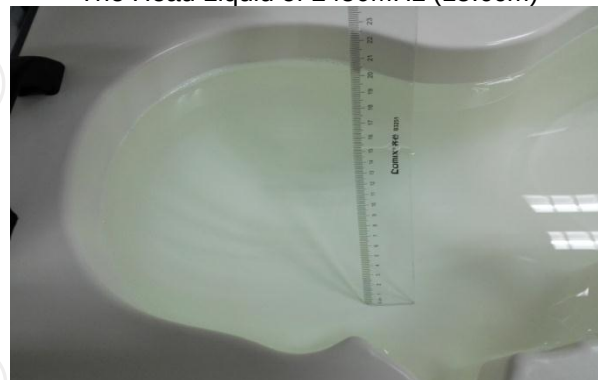
The Head Liquid of 1800MHz (15.2cm)
