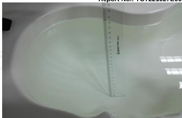
The Head Liquid of 2450MHz (15.6cm)
