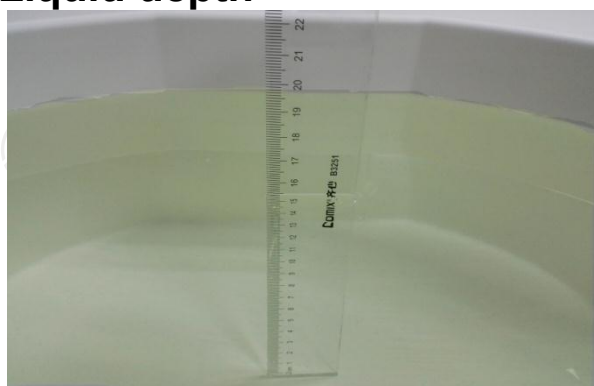
The Body Liquid of 835MHz (15.4cm)
