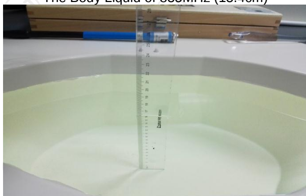
The Body Liquid of 1900MHz (16.4 cm)
