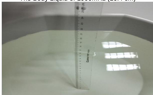
The Body Liquid of 2600MHz (16.5cm)
