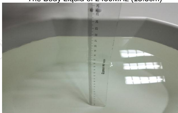
The Body Liquid of 5000-6000MHz (16.5cm)
