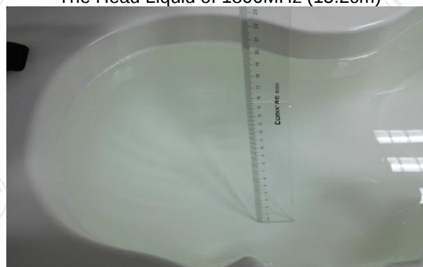
The Body Liquid of 5000-6000MHz (15.8cm)
