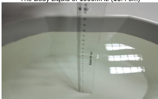
The Body Liquid of 2600MHz (16.5cm)
