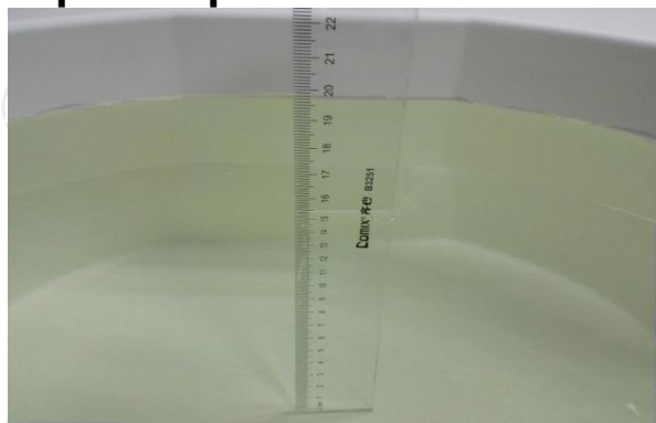
The Body Liquid of 835MHz (15.4cm)
