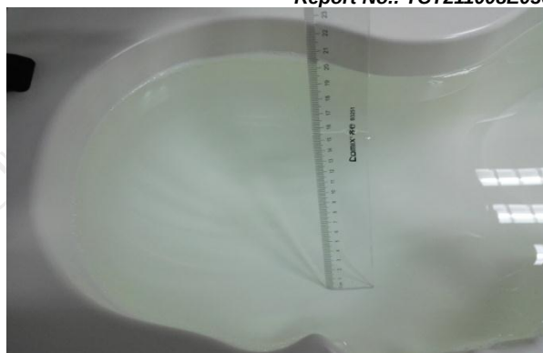
The Head Liquid of 2450MHz (15.6cm)
