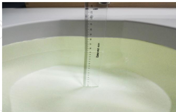
The Body Liquid of 1800MHz (15.2 cm)
