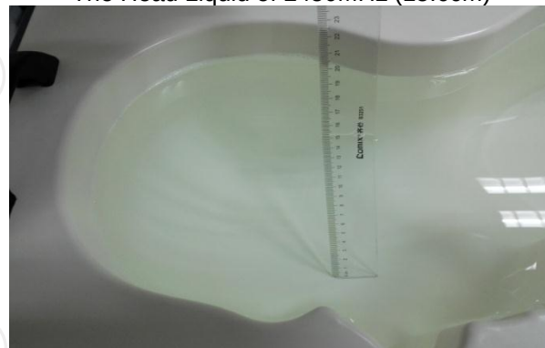
The Head Liquid of 1800MHz (15.2cm)
