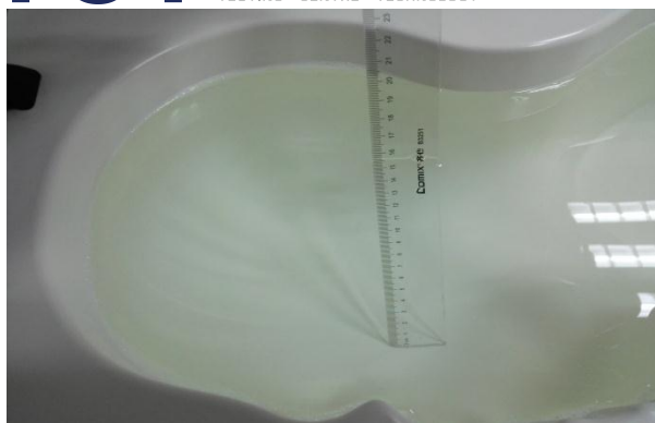
The Head Liquid of 1900MHz (15.5cm)
