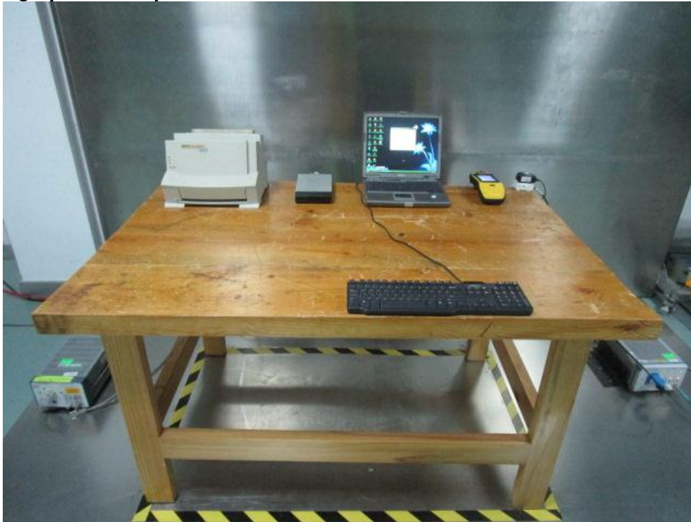
Photograph 2: Set-up for Spurious Emissions below 1GHz
