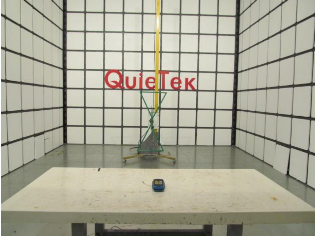
Photograph 2: Set-up for Radiated Emission, 30MHz-1000MHz
