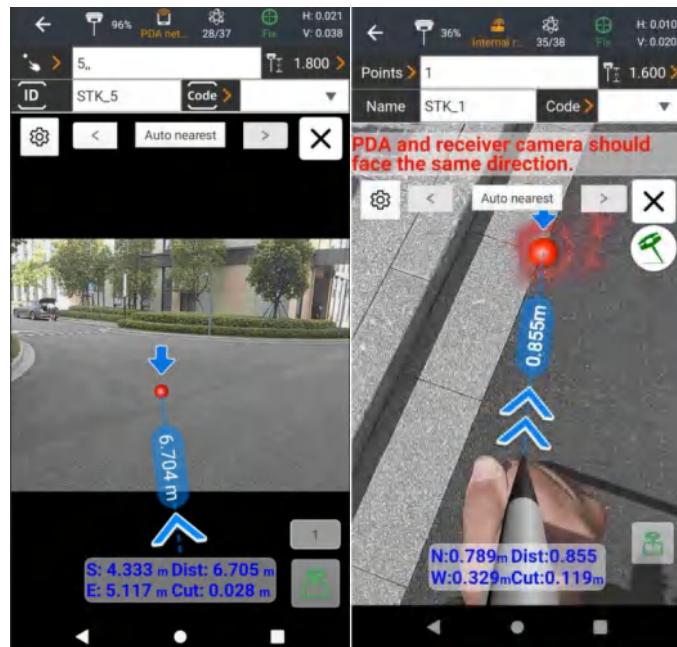
(4) In the video, the target stakeout point appears as a red dot. When the virtual pole tip touches the dot, you've reached the point. Tap the stakeout icon and the point is automatically saved.
