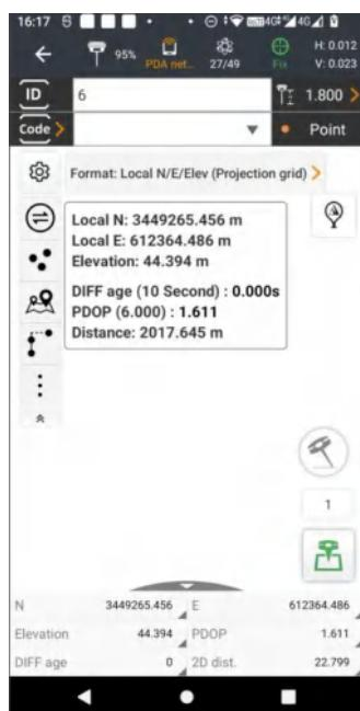
(2) Hold the pole vertical for a while and shake according to the procedures in the interface to do initialization.
