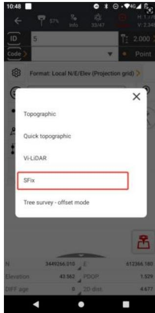
(2) The software will first enter the initialization screen. Follow the on-screen prompts to complete the initialization. Once finished, the software will automatically switch to the S-Fix point measurement screen, and S-Fix mode will be ready for use;
