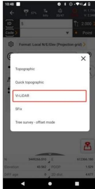
(2) The software will first enter the initialization screen. Follow the on-screen prompts to complete the initialization. Once finished, the software will automatically switch to the Vi-LiDAR point measurement screen, and Vi-LiDAR mode will be ready for use;
