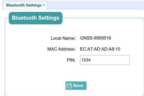
The screenshot shows the 'Bluetooth Settings' submenu. At the top, it displays the local name 'GNSS-9999516' and MAC address 'EC:A7:AD:AD:A8:10'. Below that is a text input field for the PIN, currently set to '1234'. At the bottom is a 'Save' button.
