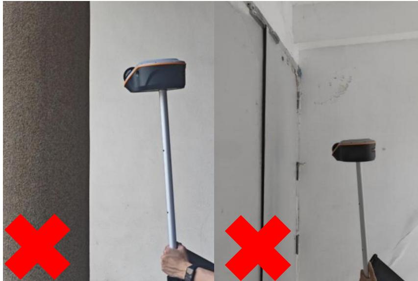
(6) In Vi-LiDAR mode, ensure no moving people or objects are in front of the camera before shooting to avoid point-cloud noise and mis-selection.
