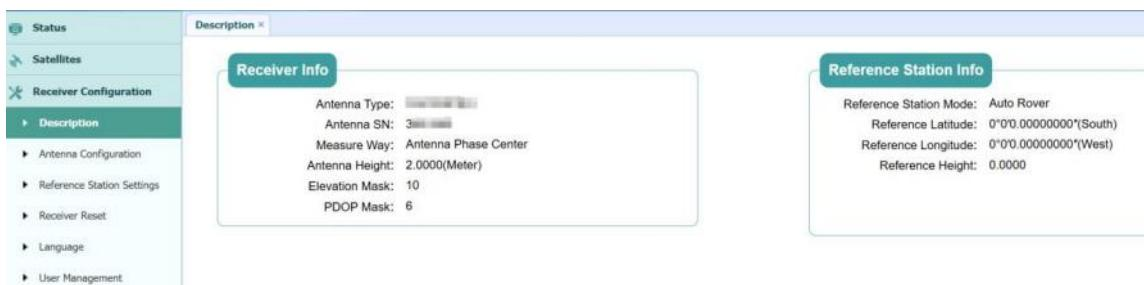
This submenu shows the receiver information and reference station information, including antenna related information, elevation mask angle, reference station work mode and position, etc.
