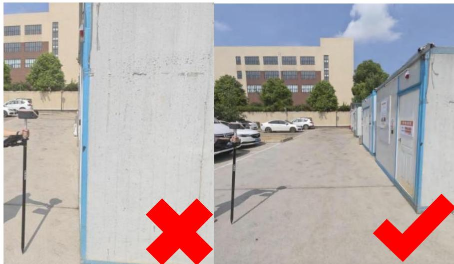
(15) Minimize fast-moving people or objects in the scene and keep the radar front clear to reduce motion noise.
