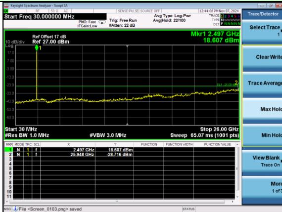
Test Mode: LTE Band 7 / 5MHz /25RB
