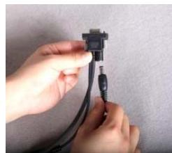
Connect the Power Adapter socket to the mains100-240 VAC and Power Adapter male connector to the Power Port of the GPS to PC cable.
