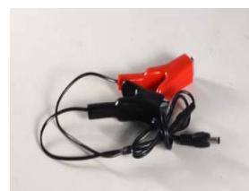
Properly connect the external power cable to a car battery (respecting the polarity) and then connect the Power Adapter male connector to the Power Port of the GPS to PC cable.
