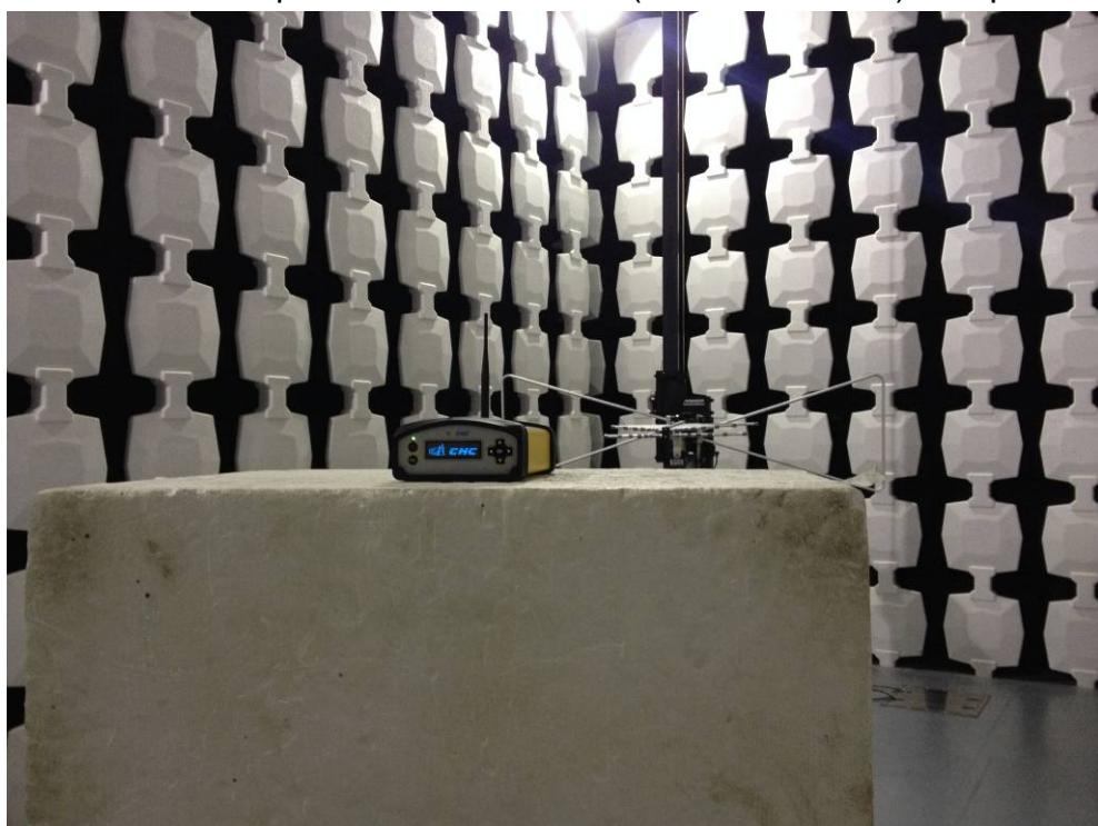
Radiated Spurious Measurement (Above 1GHz) Setup
