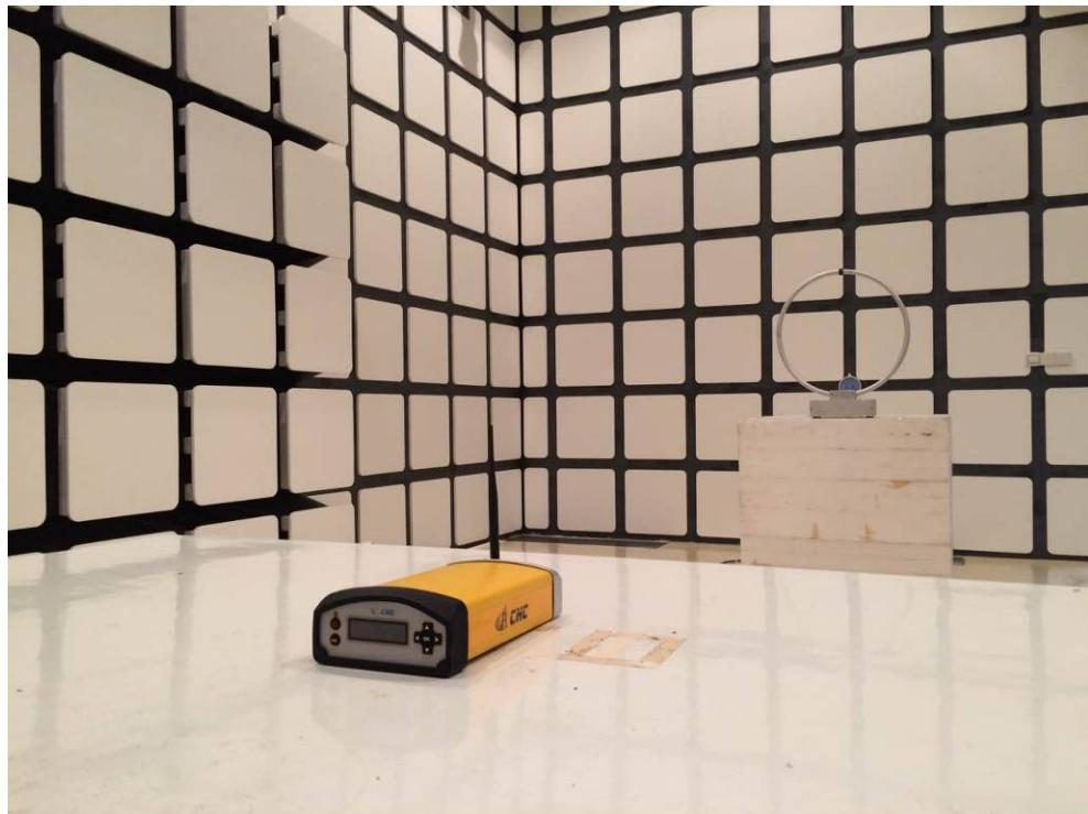
Radiated Spurious Measurement (30MHz to 1GHz) Setup
