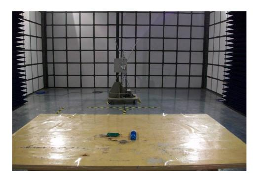
**Radiation Emission Test View For 1GHz-25GHz**
