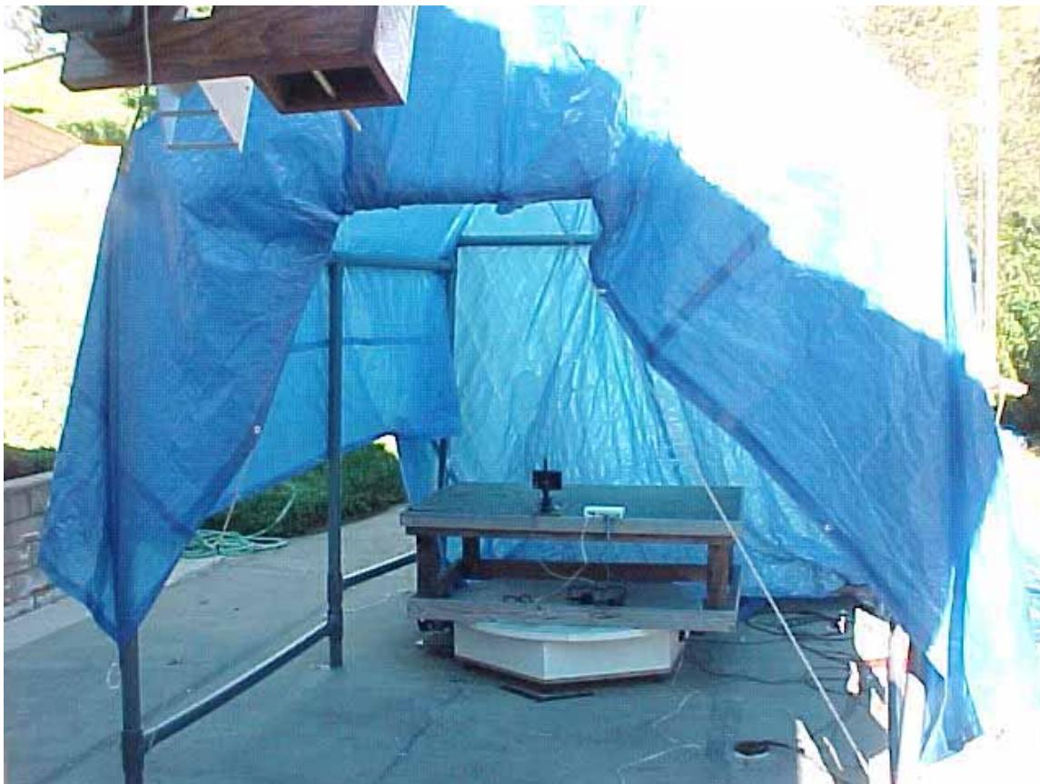
**REAR VIEW****EMBEDDED PROCESSOR DESIGNS, INC.****InfoCube BASE****MODEL: 1****FCC SUBPART B AND FCC SUBPART C – RADIATED EMISSIONS****PHOTOGRAPH SHOWING THE EUT CONFIGURATION
