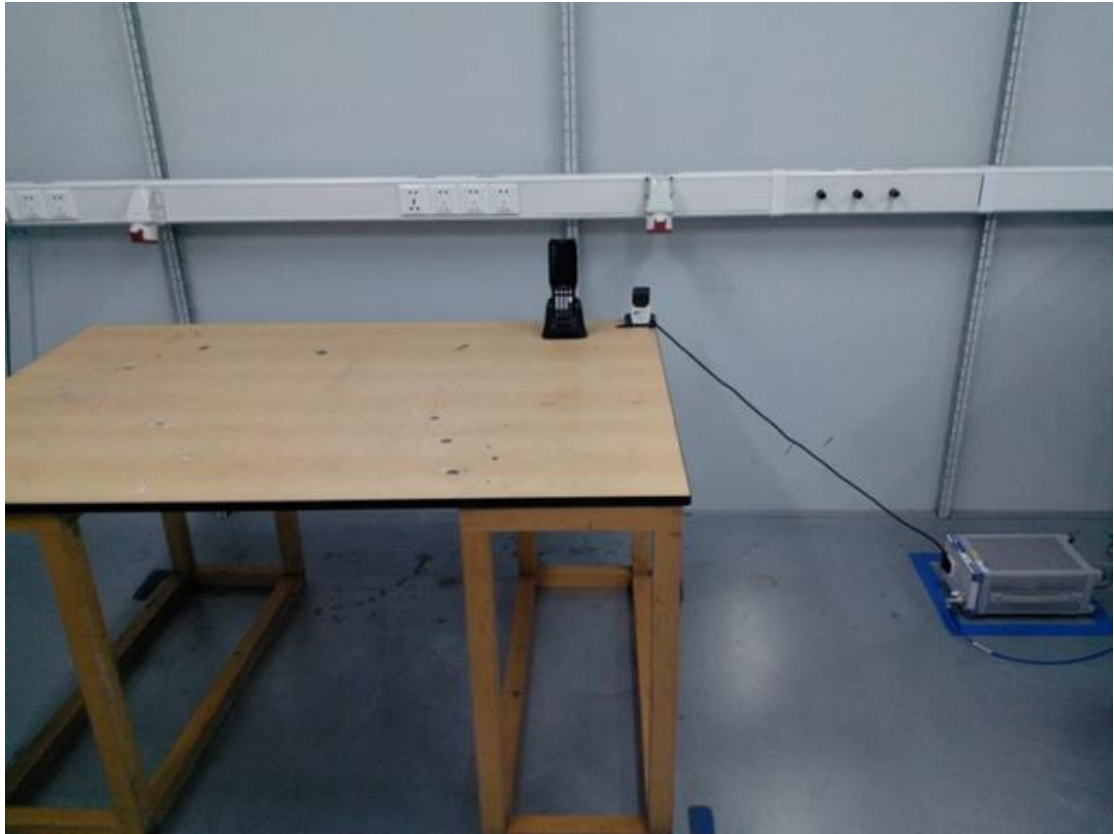
AC Conducted Emission Test Setup -Front
