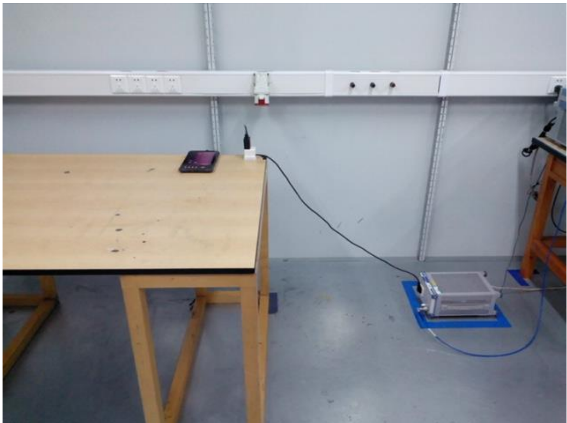
AC Conducted Emission Test Setup -Front
