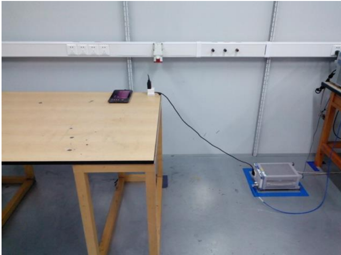
AC Conducted Emission Test Setup -Front
