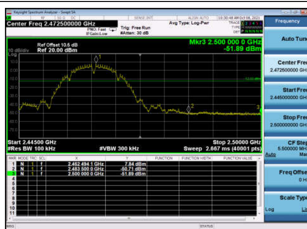
,Plot 2,Band Edge-802.11b,2462MHz ,Ant0
