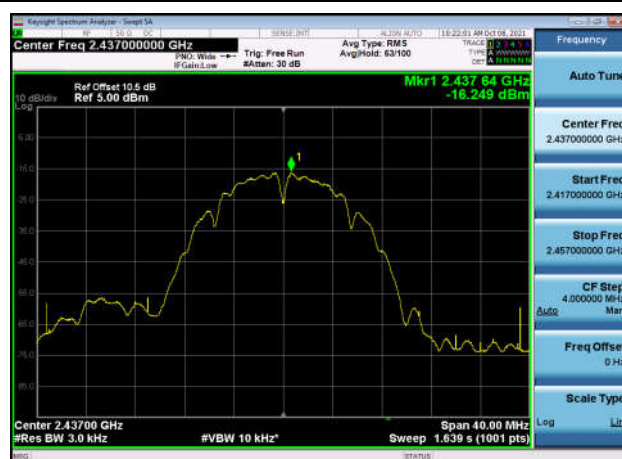
Power spectral density-802.11g ,2412MHz,Ant0
