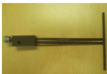
Figure 1 – MVG COMOSAR Validation Dipole
