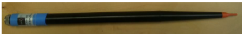
Figure 1 – MVG COMOSAR Dosimetric E field Dipole
