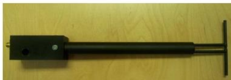
Figure 1 – MVG COMOSAR Validation Dipole
