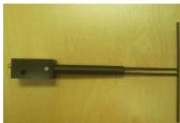
Figure 1 – MVG COMOSAR Validation Dipole
