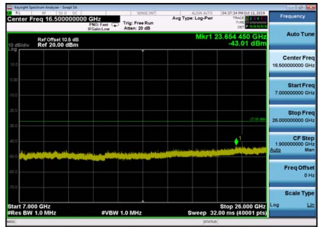
U-NII-2c ,Plot 4,7000MHz~26000MHz-802 .11a(20MHz),5700MHz,Ant2
