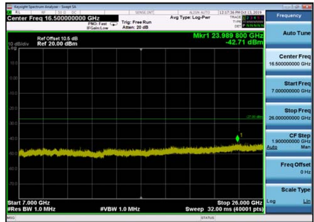
U-NII-3 ,Plot 1,Band Edge-802.11n(20M Hz),5745MHz,Ant2
