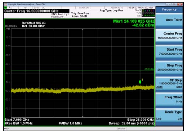
U-NII-2c ,Plot 4,7000MHz~26000MHz-802 .11n(20MHz),5700MHz,Ant2
