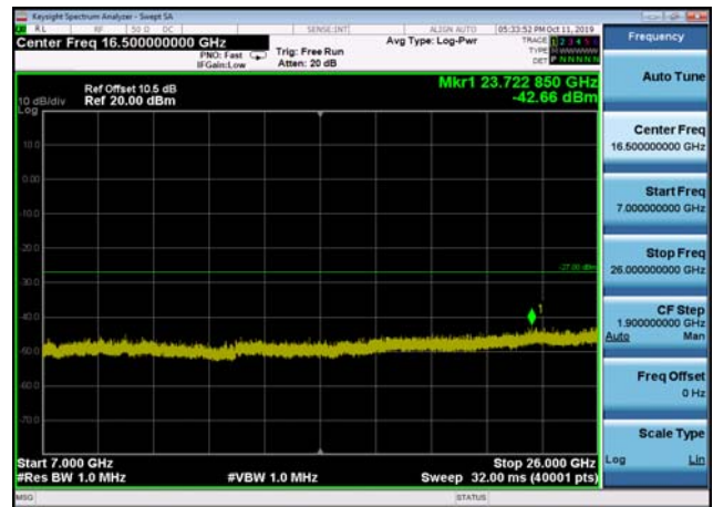
U-NII-2a ,Plot 1,Band Edge-802.11n(20 MHz),5260MHz,Ant2
