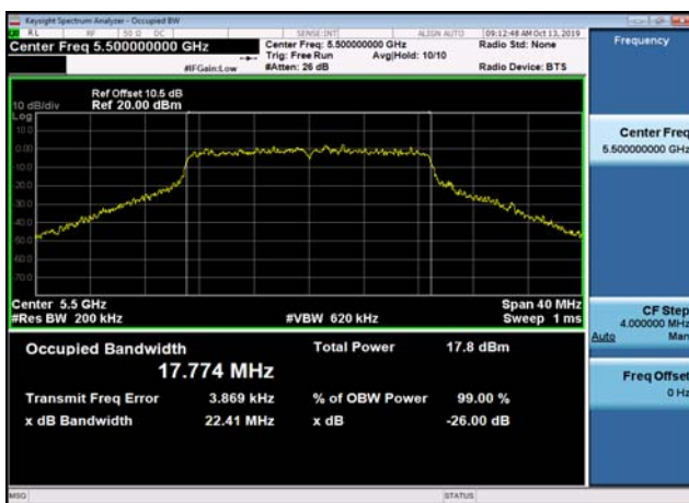
U-NII-2c 26dB Bandwidth-802.11n(20MHz),5500MHz,Ant1
