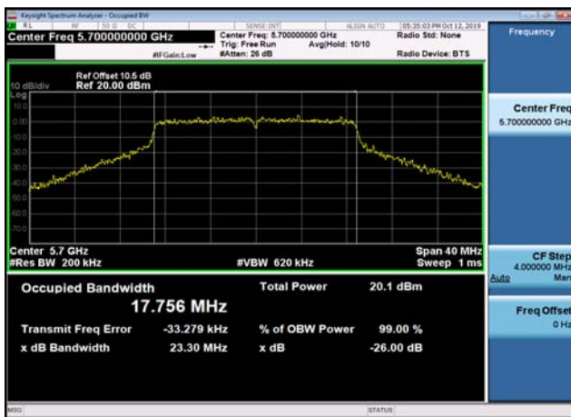
U-NII-2c 26dB Bandwidth-802.11n(40MHz) ,5510MHz,Ant1
