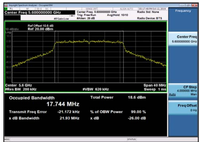
U-NII-2c 26dB Bandwidth-802.11n(20MHz) ,5700MHz,Ant2
