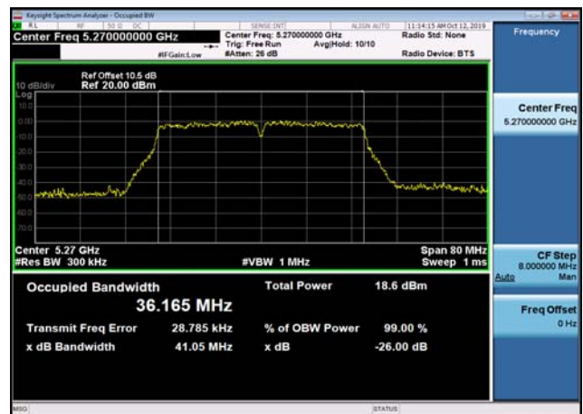
U-NII-2a 26dB Bandwidth-802.11ac(40MHz),5310MHz,Ant2
