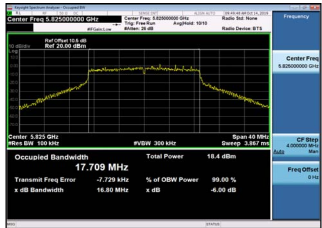
U-NII-3 6dB Bandwidth-802.11n(40MHz) ,5755MHz,Ant2
