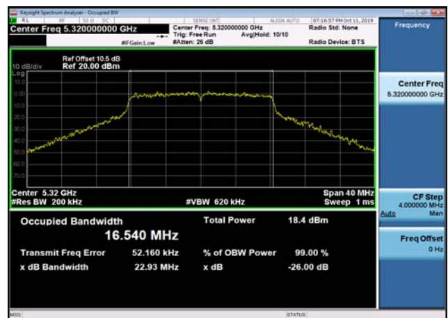
U-NII-2a 26dB Bandwidth-802.11a(20MHz ) ,5320MHz,Ant2
