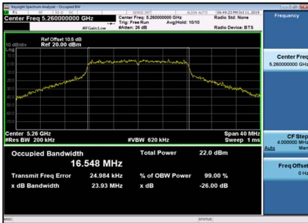
U-NII-2a 26dB Bandwidth-802.11a(20MHz ) ,5300MHz,Ant1
