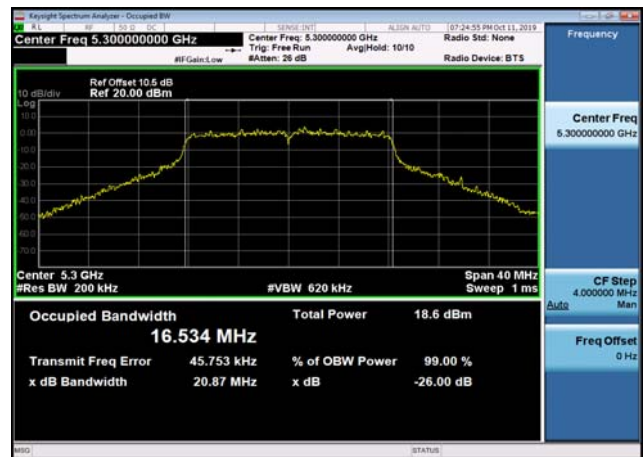
U-NII-2a 26dB Bandwidth-802.11a(20MHz ) ,5320MHz,Ant2
