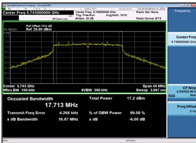
U-NII-3 6dB Bandwidth-802.11ac(20MHz) ,5785MHz,Ant1
