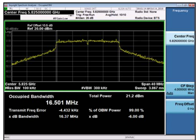
U-NII-3 6dB Bandwidth-802.11ac(20MHz) ,5745MHz,Ant2
