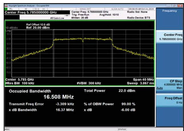
U-NII-3 6dB Bandwidth-802.11a(20MHz) ,5785MHz,Ant2
