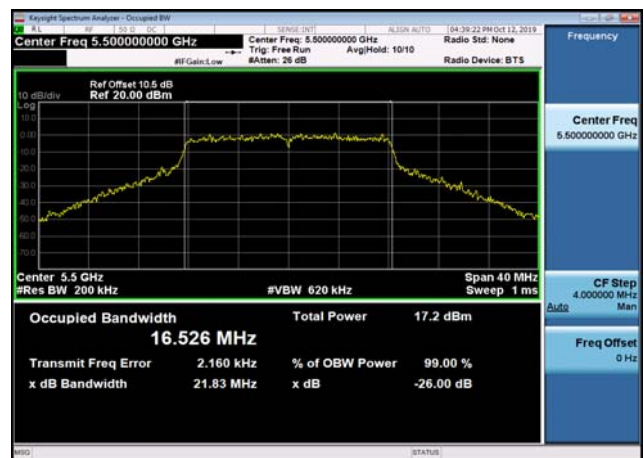
U-NII-2c 26dB Bandwidth-802.11a(20MHz) ,5500MHz,Ant2
