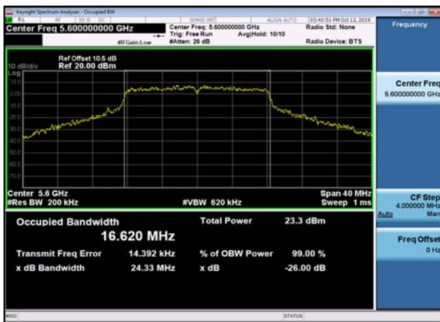
U-NII-2c 26dB Bandwidth-802.11a(20MHz ) ,5700MHz,Ant1
