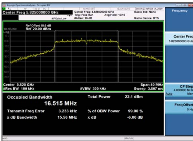
U-NII-3 6dB Bandwidth-802.11ac(20MHz) ,5745MHz,Ant1
