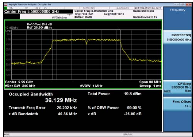
U-NII-2c 26dB Bandwidth-802.11n(40MHz) ,5670MHz,Ant2
