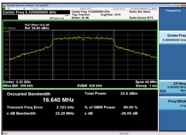
U-NII-2a 26dB Bandwidth-802.11a(20MHz ) ,5320MHz,Ant1
