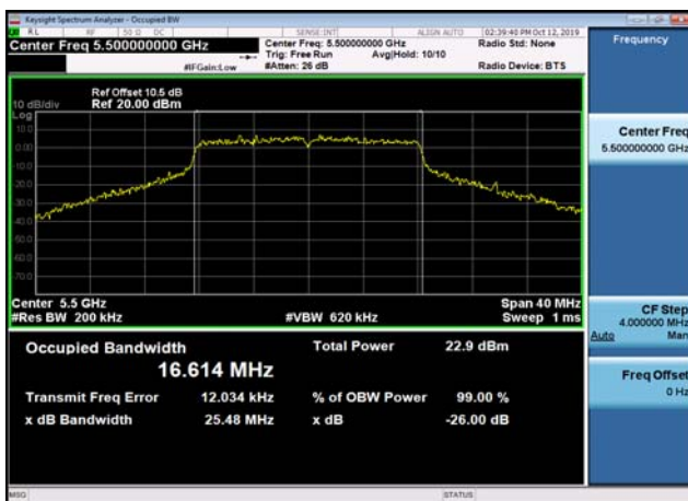
U-NII-2c 26dB Bandwidth-802.11a(20MHz) ,5500MHz,Ant1
