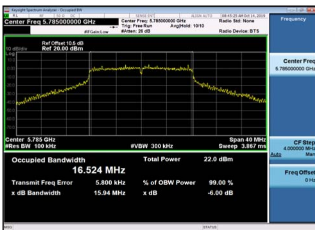
U-NII-3 6dB Bandwidth-802.11a(20MHz) ,5785MHz,Ant1
