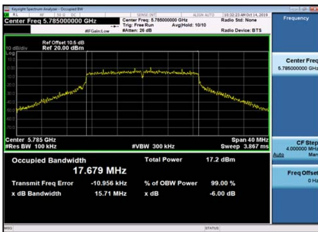
U-NII-3 6dB Bandwidth-802.11ac(20MHz) ,5785MHz,Ant1
