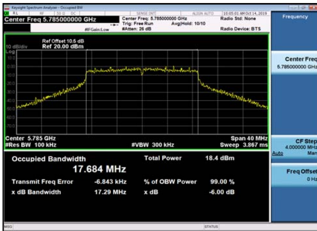
U-NII-3 6dB Bandwidth-802.11n(20MHz) ,5825MHz,Ant1
