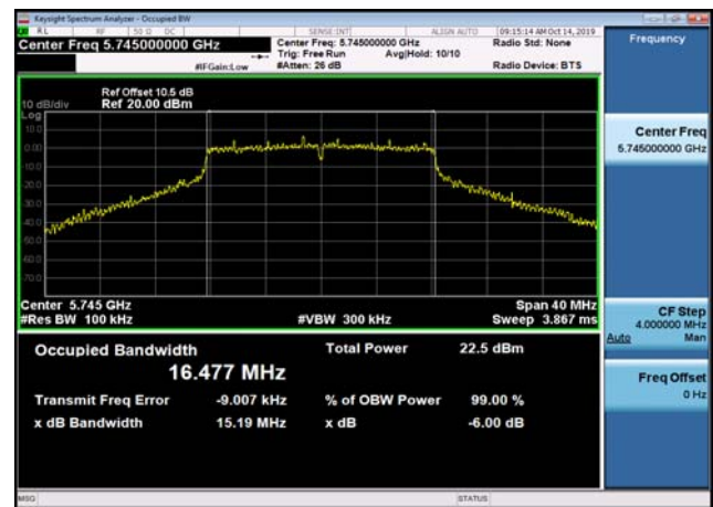
U-NII-3 6dB Bandwidth-802.11a(20MHz) ,5785MHz,Ant2
