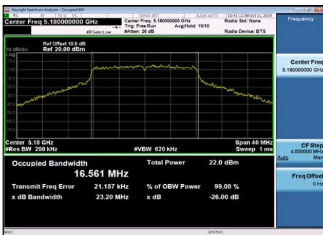
U-NII-1 26dB Bandwidth-802.11a(20MHz) ,5180MHz,Ant1
