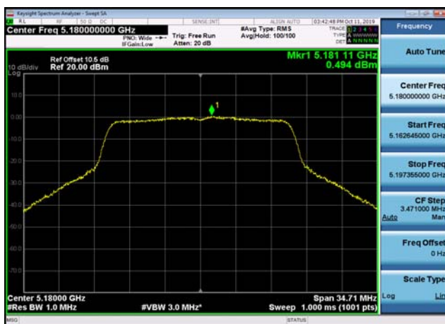
U-NII-1 Power spectral density-802.11 ac(20MHz),5180MHz,Ant1
