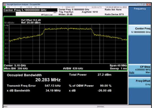
U-NII-1 26dB Bandwidth-802.11a(20MHz) ,5180MHz,Ant2
