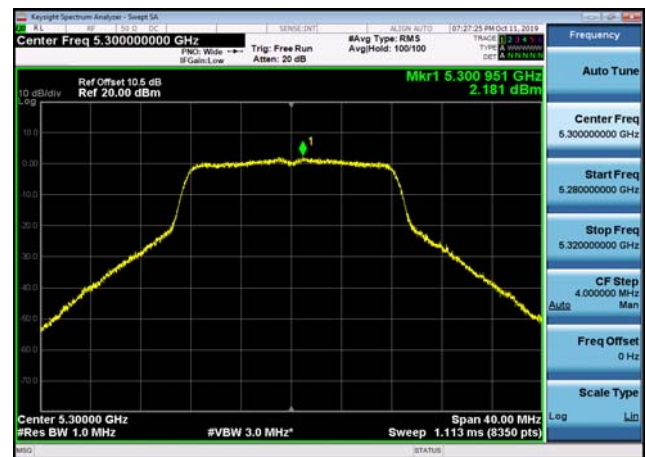
U-NII-2a Power spectral density-802.1 1a(20MHz),5320MHz,Ant2
