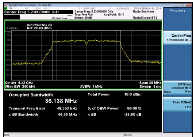
U-NII-1 26dB Bandwidth-802.11a(20MHz) ,5180MHz,Ant2
