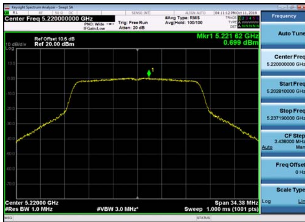
U-NII-1 Power spectral density-802.11 ac(20MHz),5240MHz,Ant1
