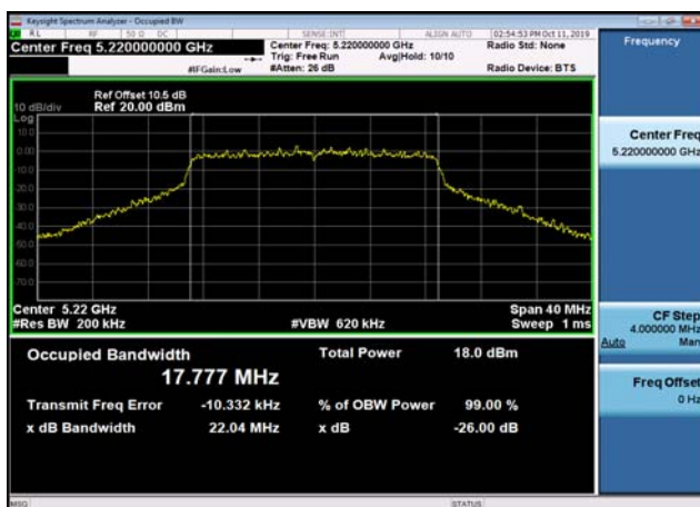
U-NII-1 26dB Bandwidth-802.11n(20MHz) ,5240MHz,Ant1
