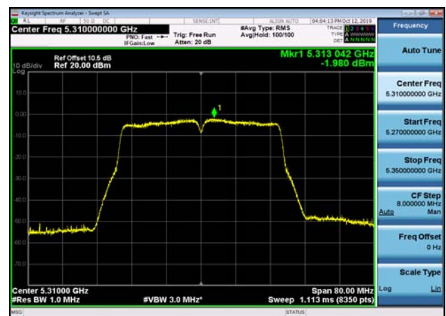
U-NII-2a Power spectral density-802.1 1n(40MHz),5310MHz,Ant2
