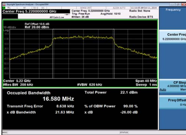
U-NII-1 26dB Bandwidth-802.11a(20MHz) ,5240MHz,Ant1
