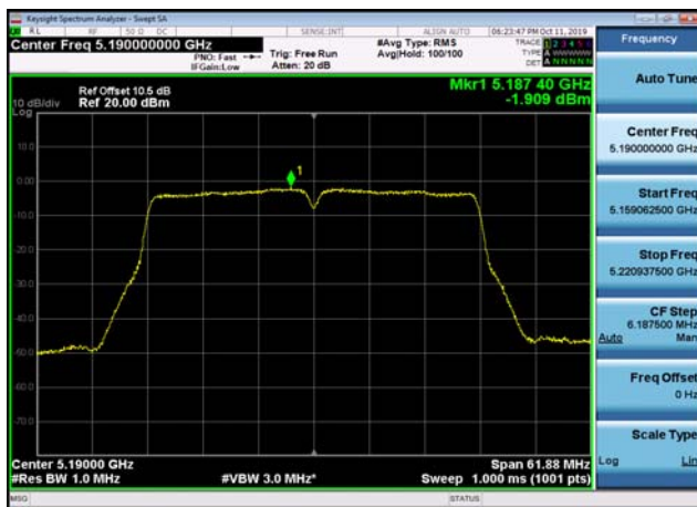
U-NII-1 Power spectral density-802.11 ac(40MHz),5190MHz,Ant1
