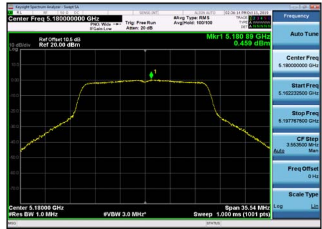
U-NII-1 Power spectral density-802.11 n(20MHz),5220MHz,Ant2
