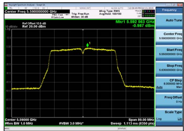
U-NII-2c Power spectral density-802.1 1ac(40MHz),5670MHz,Ant2
