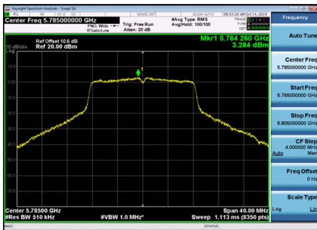
U-NII-3 Power spectral density-802.11 a(20MHz),5785MHz,Ant1
