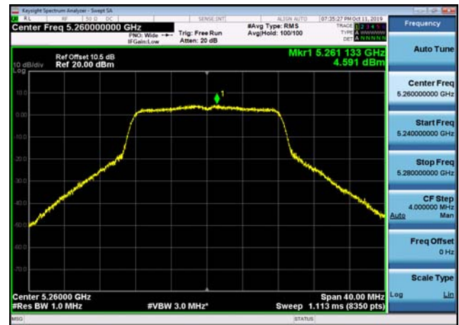
U-NII-2a Power spectral density-802.1 1a(20MHz),5300MHz,Ant2
