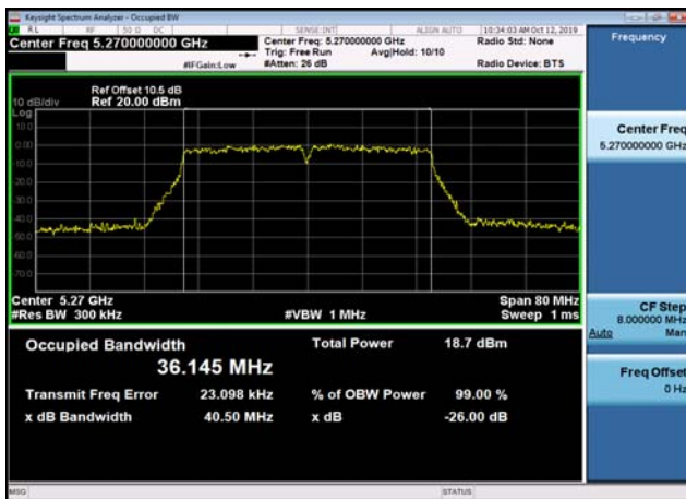
U-NII-2a 26dB Bandwidth-802.11n(40MHz ,5310MHz,Ant1
