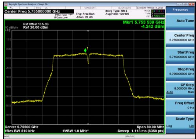
U-NII-3 Power spectral density-802.11 ac(40MHz),5795MHz,Ant2
