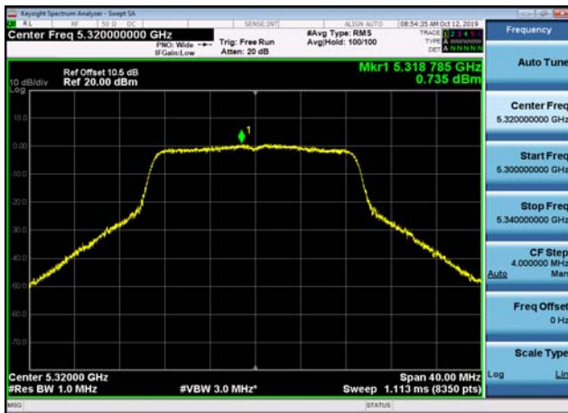
U-NII-2a Power spectral density-802.1 1n(40MHz),5270MHz,Ant1
