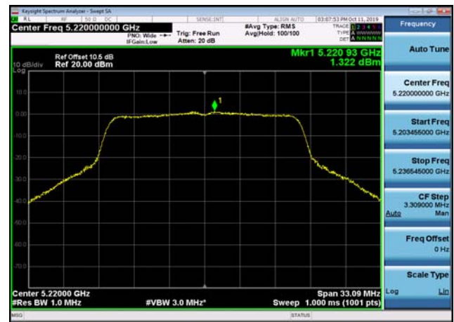
U-NII-1 Power spectral density-802.11 n(20MHz),5240MHz,Ant2
