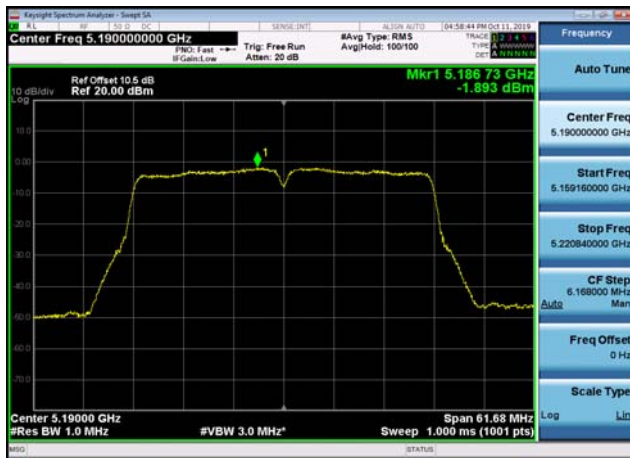
U-NII-1 Power spectral density-802.11 n(40MHz),5230MHz,Ant1
