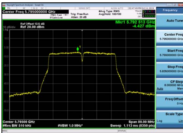
U-NII-3 Power spectral density-802.11 ac(40MHz),5795MHz,Ant1
