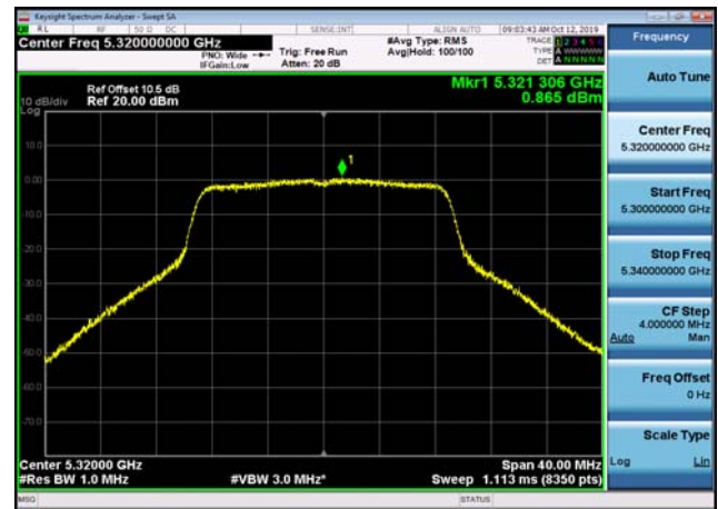
U-NII-2a Power spectral density-802.1 1n(40MHz),5270MHz,Ant2
