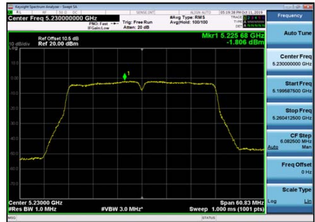
U-NII-1 Power spectral density-802.11 a(20MHz),5180MHz,Ant2
