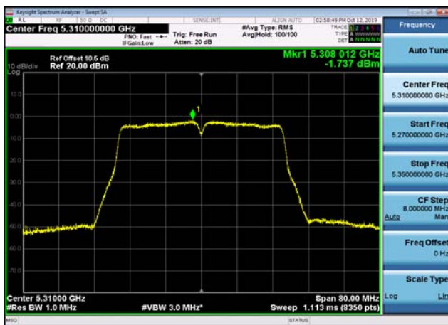
U-NII-2c Power spectral density-802.1 1n(20MHz),5500MHz,Ant1
