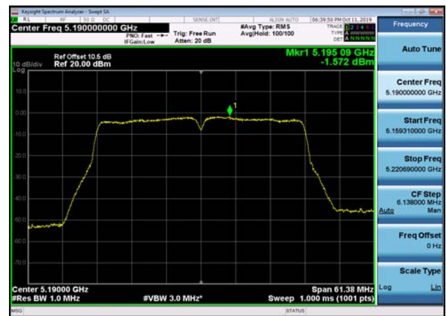
U-NII-1 Power spectral density-802.11 ac(40MHz),5190MHz,Ant2
