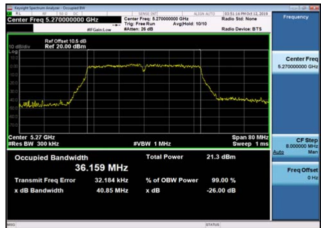
U-NII-2a 26dB Bandwidth-802.11n(40MHz ,5310MHz,Ant2
