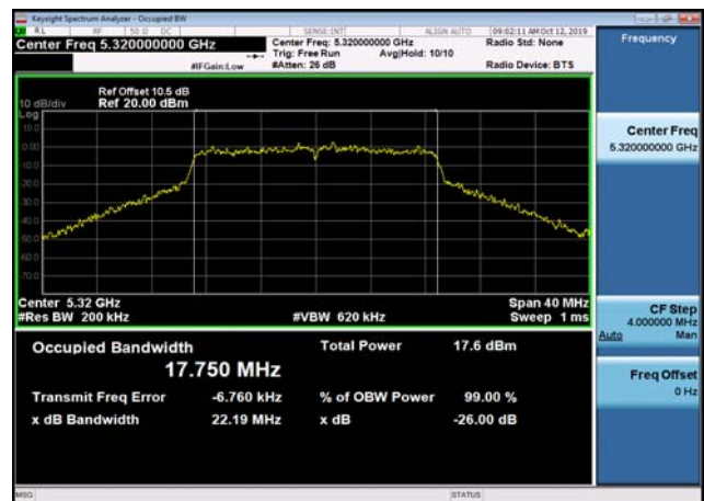
U-NII-2a 26dB Bandwidth-802.11n(40MHz ,5270MHz,Ant2
