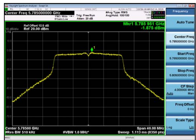
U-NII-3 Power spectral density-802.11 ac(20MHz),5785MHz,Ant2
