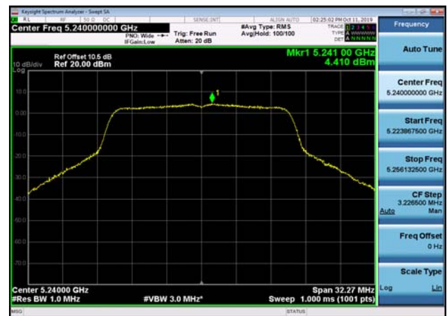
U-NII-1 Power spectral density-802.11 ac(20MHz),5180MHz,Ant2
