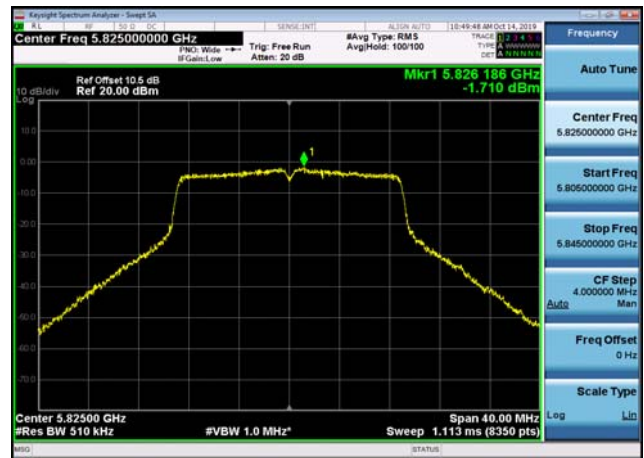
U-NII-3 Power spectral density-802.11 ac(40MHz),5755MHz,Ant2
