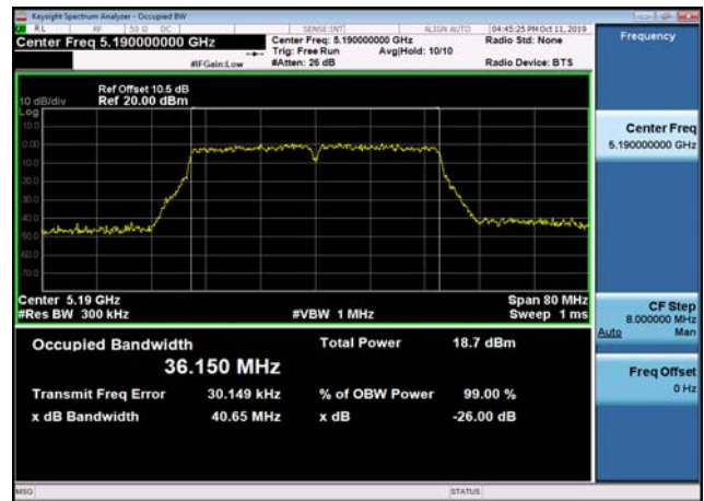
U-NII-1 26dB Bandwidth-802.11n(40MHz) ,5230MHz,Ant2
