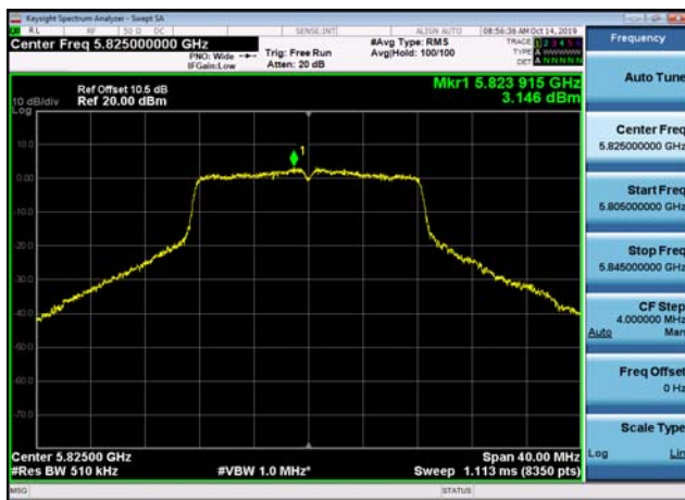
U-NII-3 Power spectral density-802.11 ac(20MHz),5745MHz,Ant1
