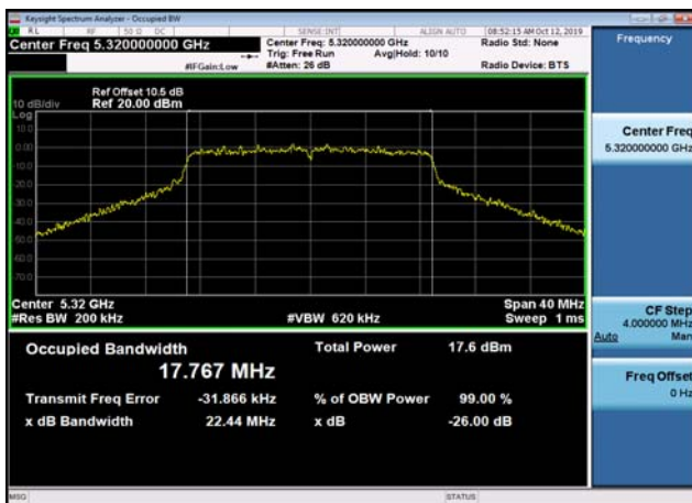
U-NII-2a 26dB Bandwidth-802.11n(40MHz ,5270MHz,Ant1
