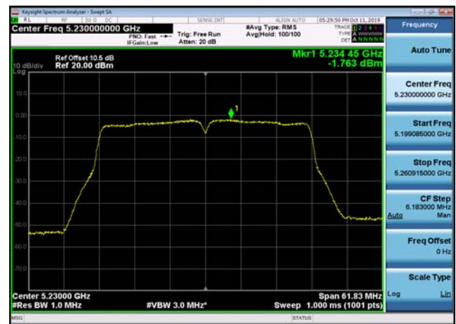
U-NII-2a Power spectral density-802.1 1n(20MHz),5260MHz,Ant2
