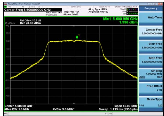
U-NII-2c Power spectral density-802.1 1a(20MHz),5700MHz,Ant2
