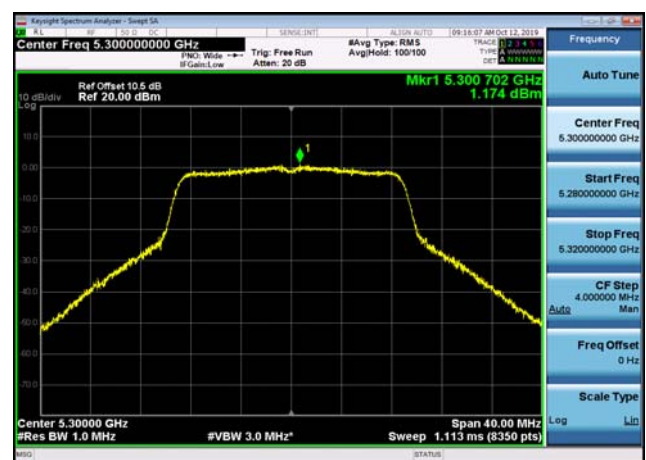
U-NII-2a Power spectral density-802.1 1n(20MHz),5300MHz,Ant2
