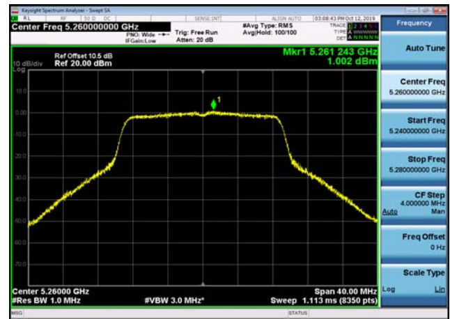
U-NII-2a Power spectral density-802.1 1ac(20MHz),5300MHz,Ant2
