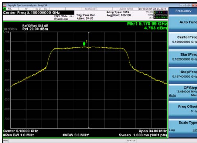
U-NII-1 Power spectral density-802.11 a(20MHz),5180MHz,Ant1
