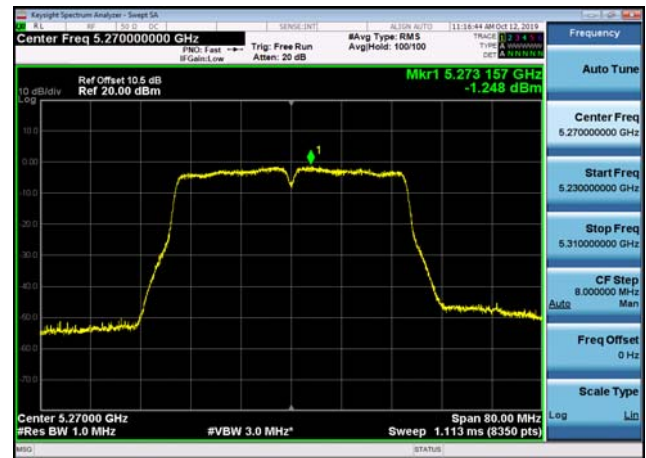
U-NII-2a Power spectral density-802.1 1ac(40MHz),5310MHz,Ant2
