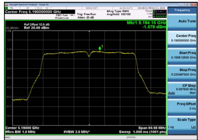
U-NII-1 Power spectral density-802.11 n(40MHz),5230MHz,Ant2
