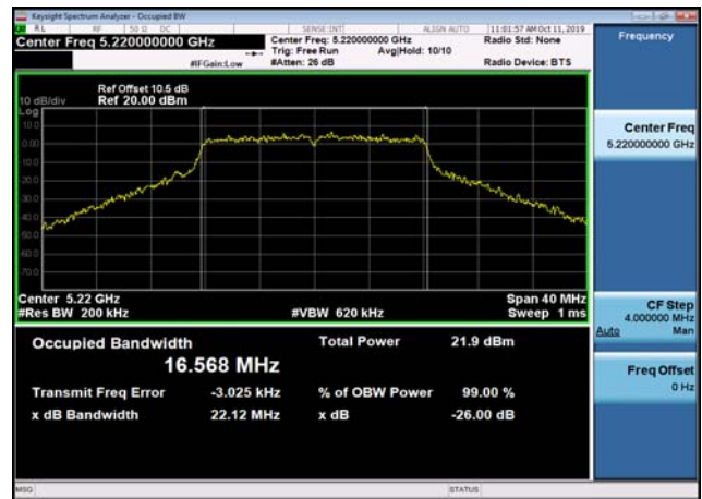
U-NII-1 26dB Bandwidth-802.11a(20MHz) ,5240MHz,Ant2
