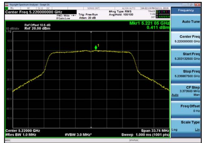
U-NII-1 Power spectral density-802.11 ac(20MHz),5240MHz,Ant2
