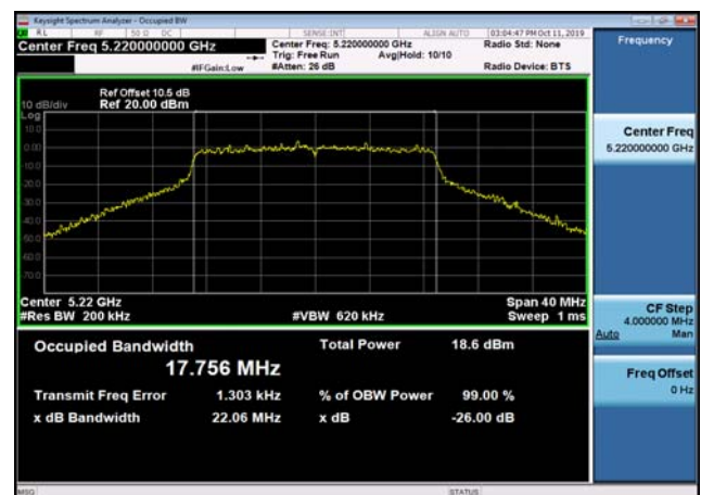
U-NII-1 26dB Bandwidth-802.11n(20MHz) ,5240MHz,Ant2
