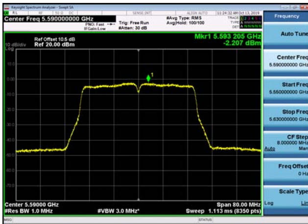
U-NII-2c Power spectral density-802.1 1n(40MHz),5670MHz,Ant1
