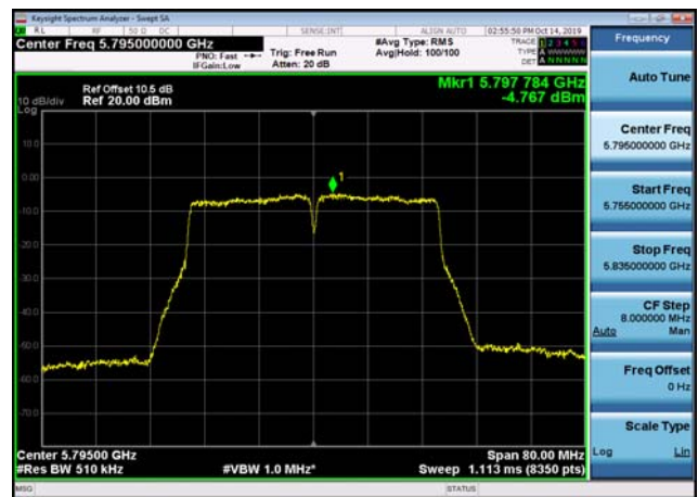
U-NII-3 Power spectral density-802.11 ac(40MHz),5795MHz,Ant2
