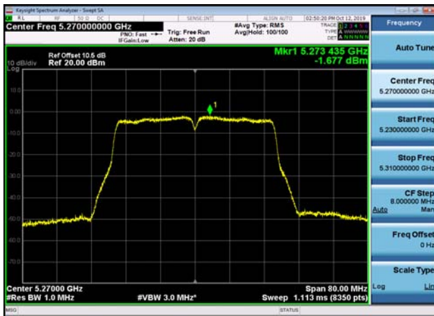
U-NII-2a Power spectral density-802.1 1ac(40MHz),5310MHz,Ant1
