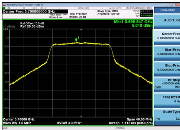
U-NII-2c Power spectral density-802.1 1ac(20MHz),5500MHz,Ant1
