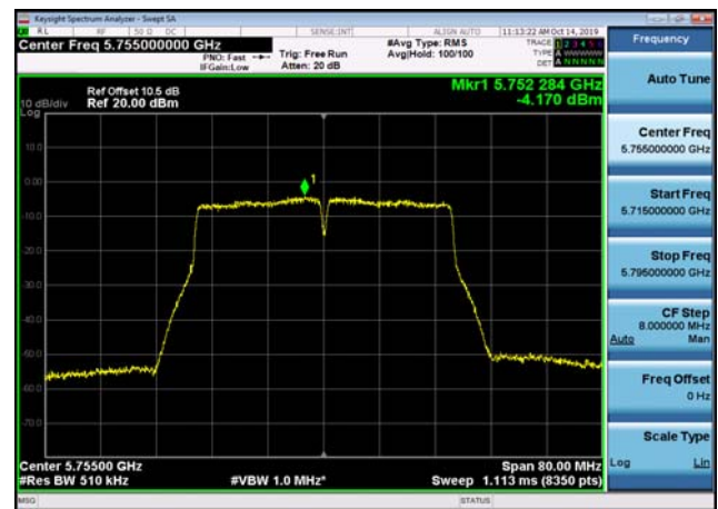
U-NII-3 Power spectral density-802.11 n(40MHz),5755MHz,Ant2
