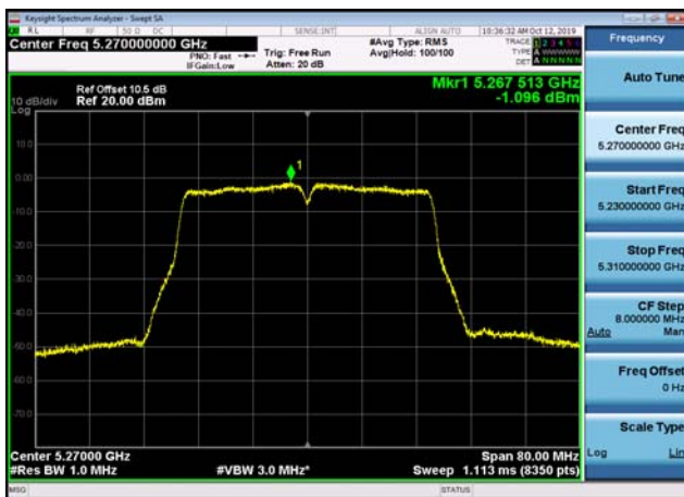
U-NII-2a Power spectral density-802.1 1n(40MHz),5310MHz,Ant1
