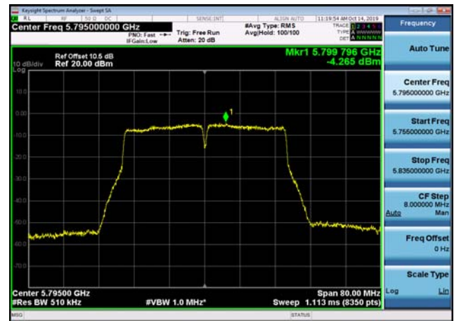
U-NII-3 Power spectral density-802.11 a(20MHz),5745MHz,Ant2
