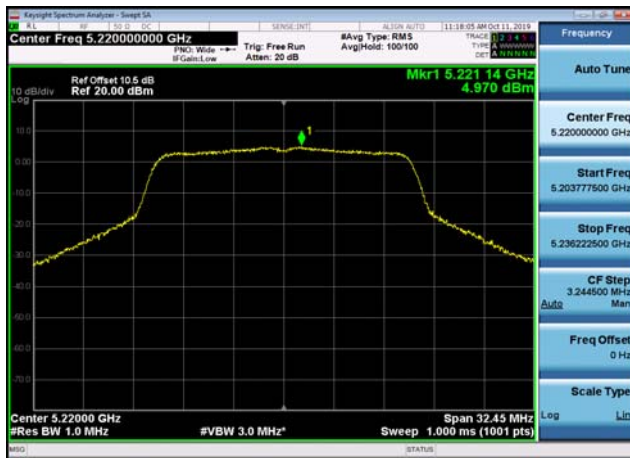
U-NII-1 Power spectral density-802.11 a(20MHz),5240MHz,Ant1
